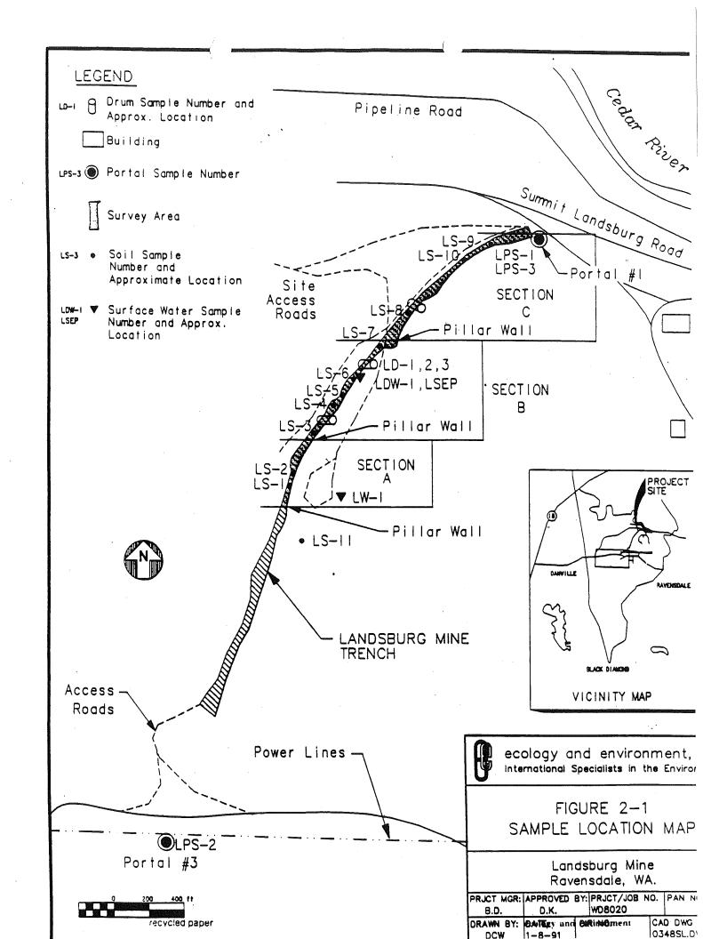
divided from the southern portion by a pillar wall. Each section of the study area also is separated by a pillar wall (Figure 2-1).
