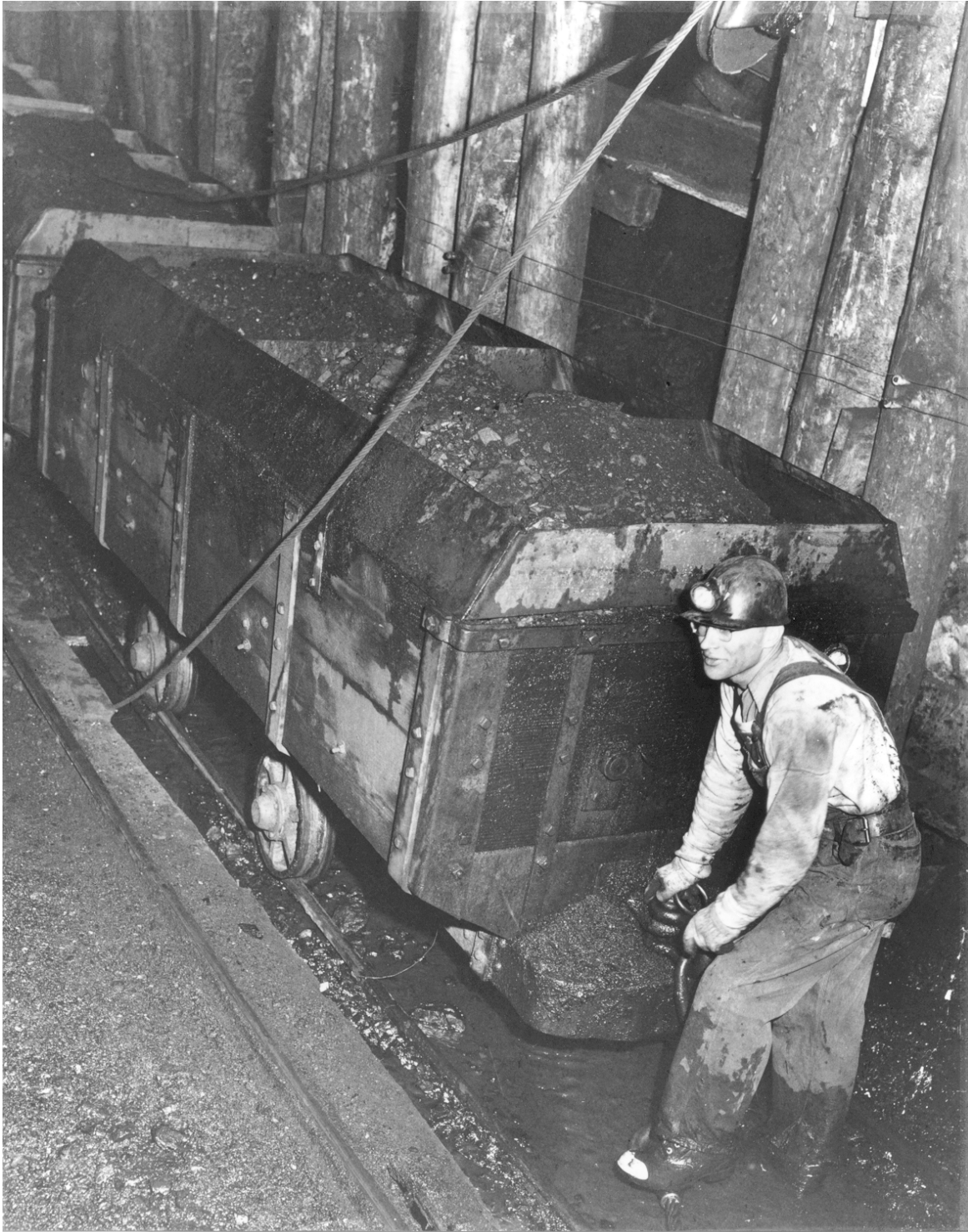
Bill McLoughry hitches another coal car to the main hoisting cable. After the cable is attached, the coal car will be pulled 500 feet up an incline to the surface. Hoisting machinery at the Landsburg Mine pulled the cars one at a time with a 125 horsepower electrical motor. circa 1953. Photograph by the Seattle Times copyright 1978 Seattle Times P.O. Box 70, Seattle, WA 98111 all rights reserved; (206) 464-229.7 This picture has been purchased for personal use only and must not be published, reproduced, or used for advertising purposes without written permission from the Seattle Times.
