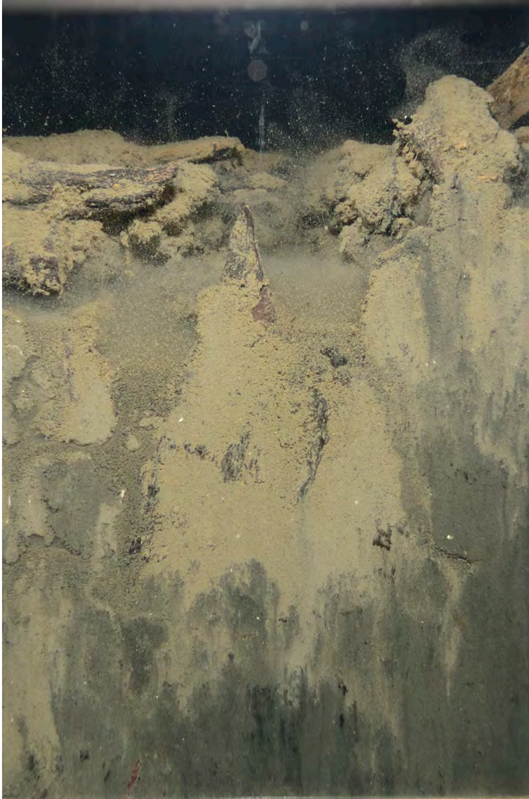
Figure 11: The disturbed sediment water interface in this profile image from Station WPAH012 is due to the camera prism dragging down some surface wood debris, resulting in a high measured value for boundary roughness. Scale: width of profile image = 14.4. cm.
