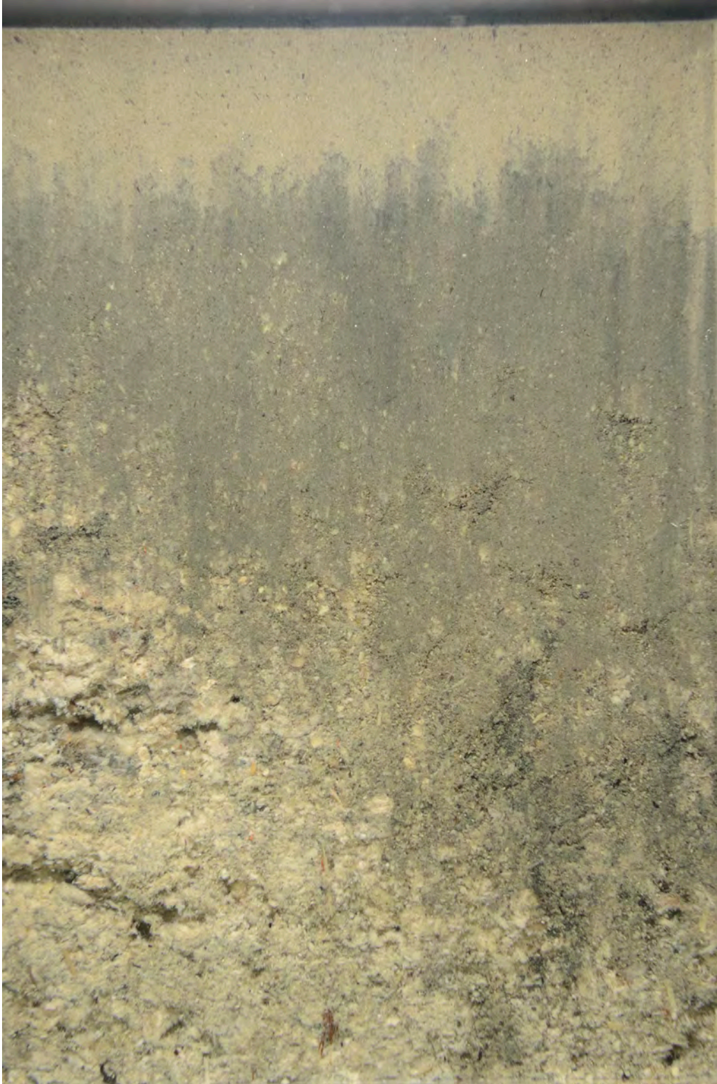
Figure 18: Even though the sediment surface cannot be seen in this profile image from Station WPAH010 where the camera over-penetrated, the “cottage cheese” texture of the pocket of wood pulp at depth is quite evident in this image. Scale: width of profile image = 14.4 cm.
