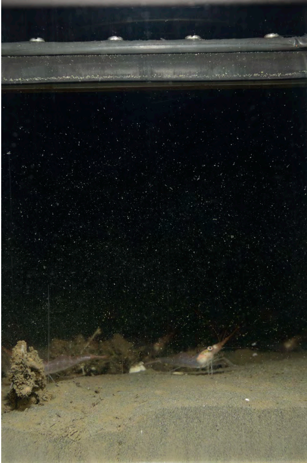
Figure 9: Despite the profile camera having the stop collars set at the maximum height and all the lead (250 lbs) in the weight carriages, the compact, very fine sand at Station WPAH047 only allowed minimal (2.06 cm) prism penetration. Scale: width of profile image = 14.4 cm.
