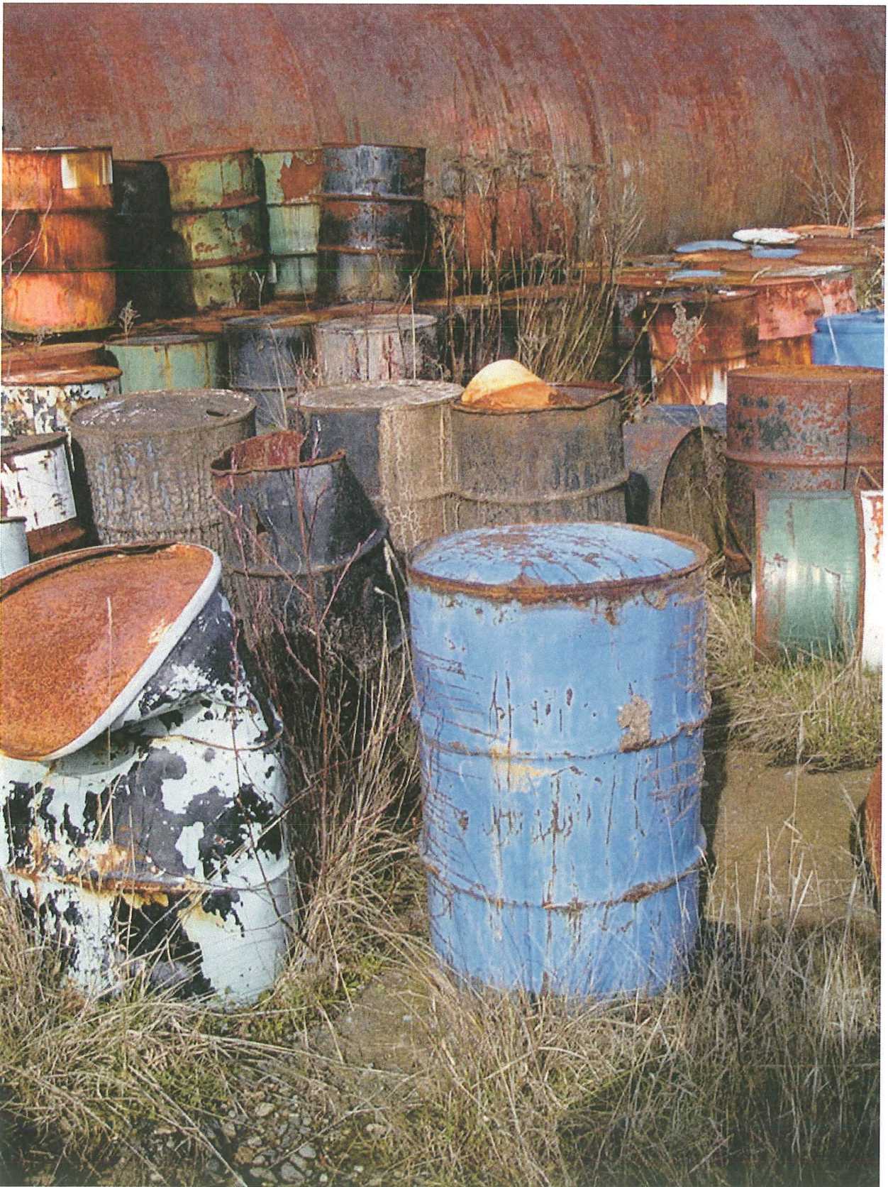
Treoil7: Detail of drums shown in Treoil6a, and spillage to the ground from drum leakage. Note bulging and leaking drums. View is towards the northwest.
