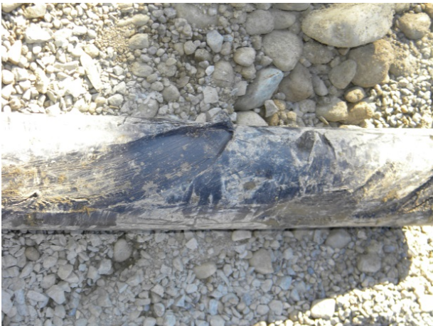
Leachate Force Main. Repaired damage to 4-inch diameter leachate force main.
