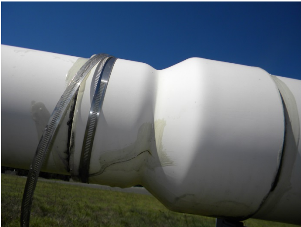
N-64B and N-64C. Fractured PVC reducer located between wells N33 and N35.
