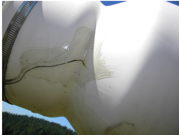
N-64B and N-64C. Fractured PVC reducer located between wells N33 and N35.
