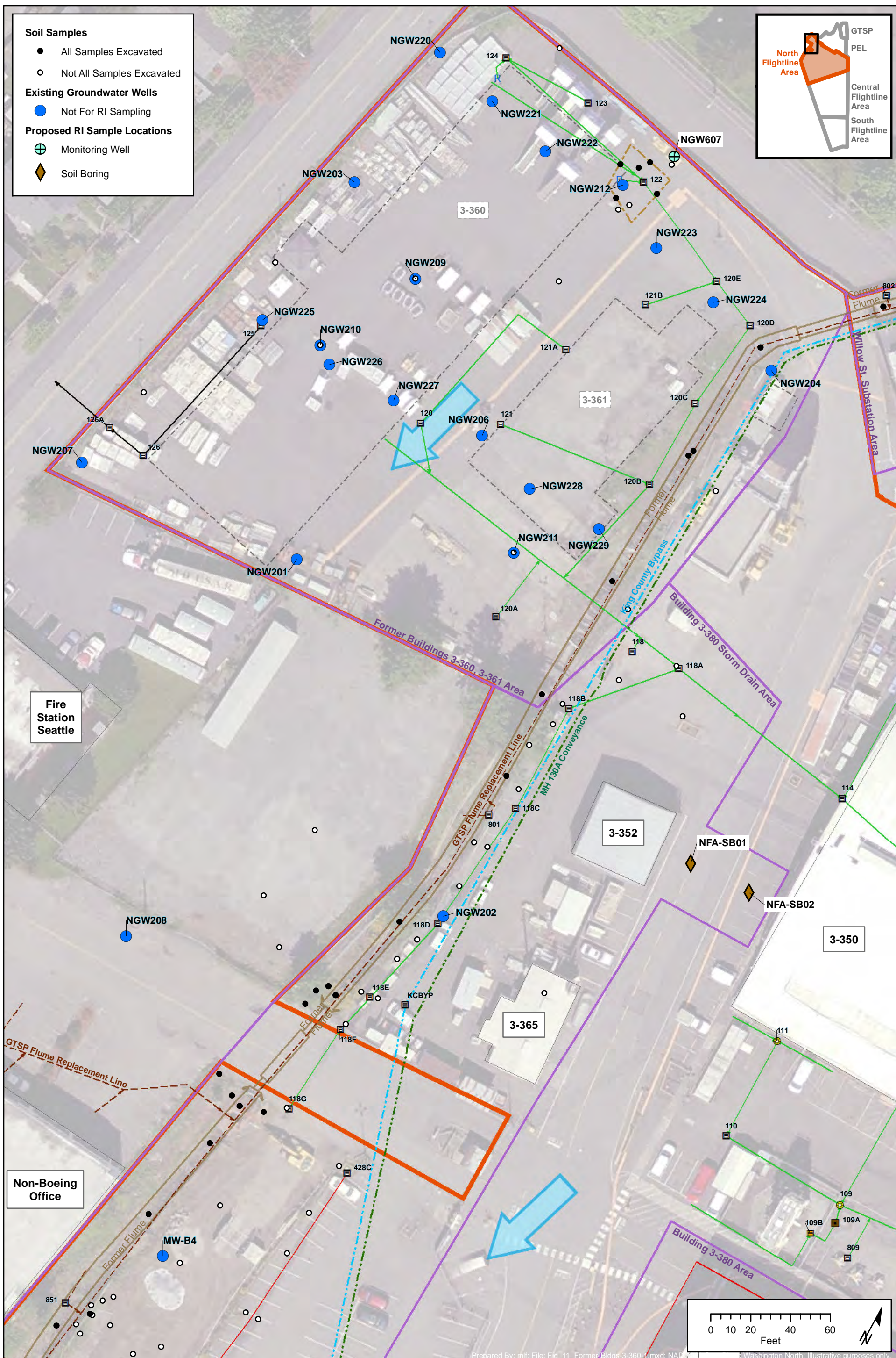
Figure 11. Proposed Soil and Groundwater Sample Locations at Former Buildings 3-360 and 3-361 Area and Building 3-380 Storm Drain Area
