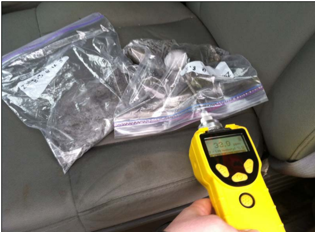
Photo 4. Field PID screening of samples from exploration B-3.
