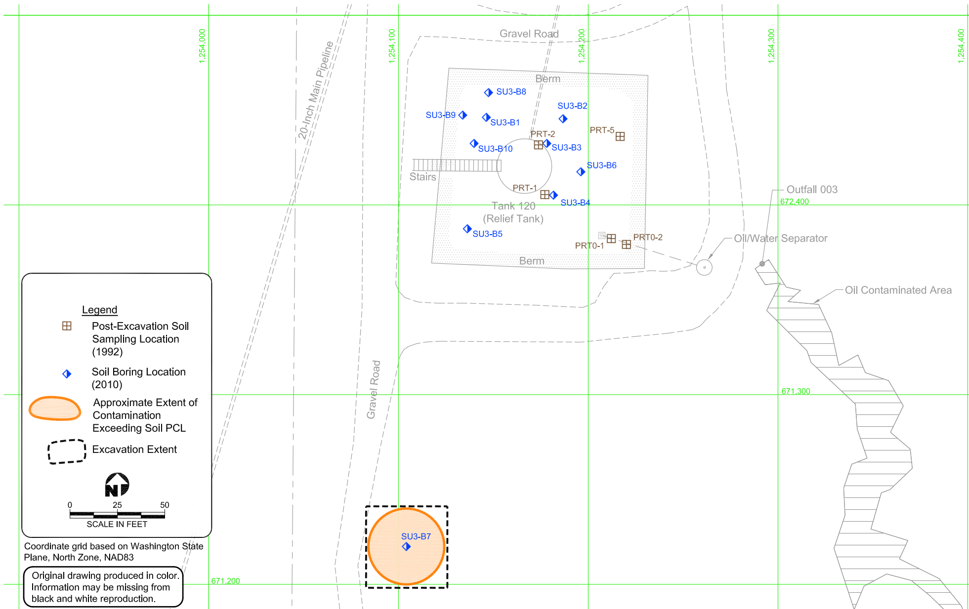
Figure 6 Excavation Extent for Material Storage Area (SU3-B7)
