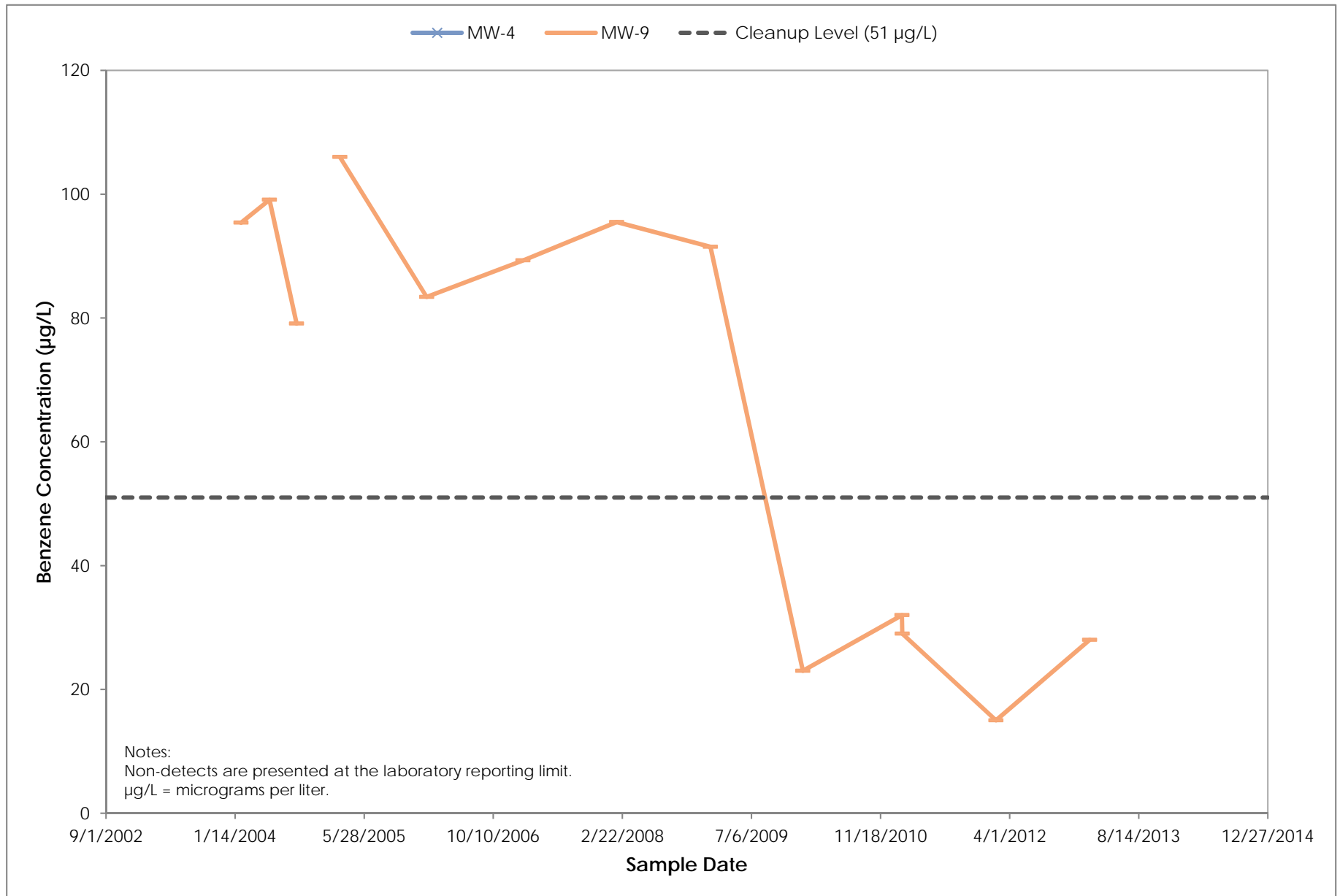
Figure 5-8 Shallow Groundwater Benzene Trend Plot (2004 to 2013) Cascade Pole and Lumber Company, Tacoma Facility Tacoma, Washington
