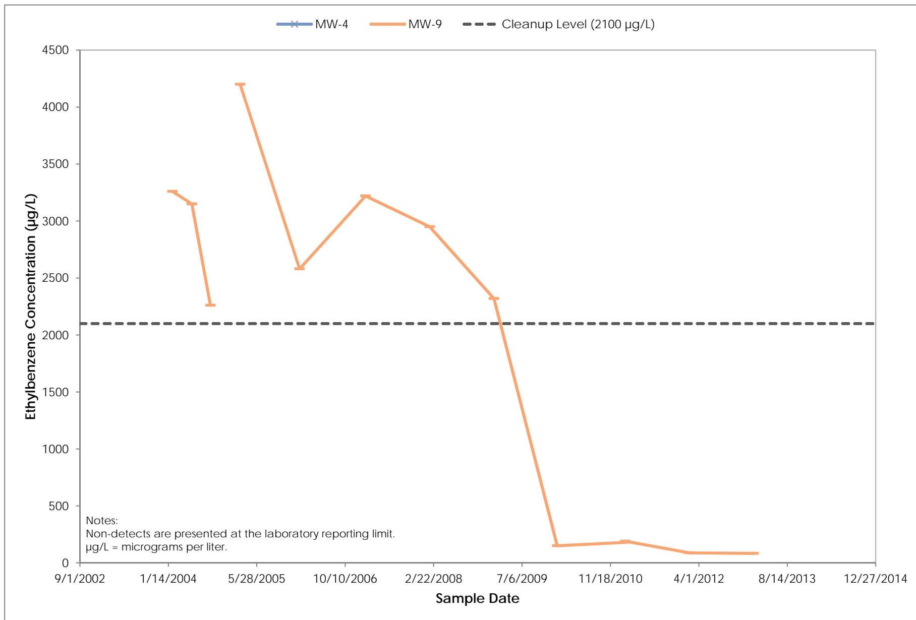
Figure 5-9 Shallow Groundwater Ethylbenzene Trend Plot (2004 to 2013) Cascade Pole and Lumber Company, Tacoma Facility Tacoma, Washington
