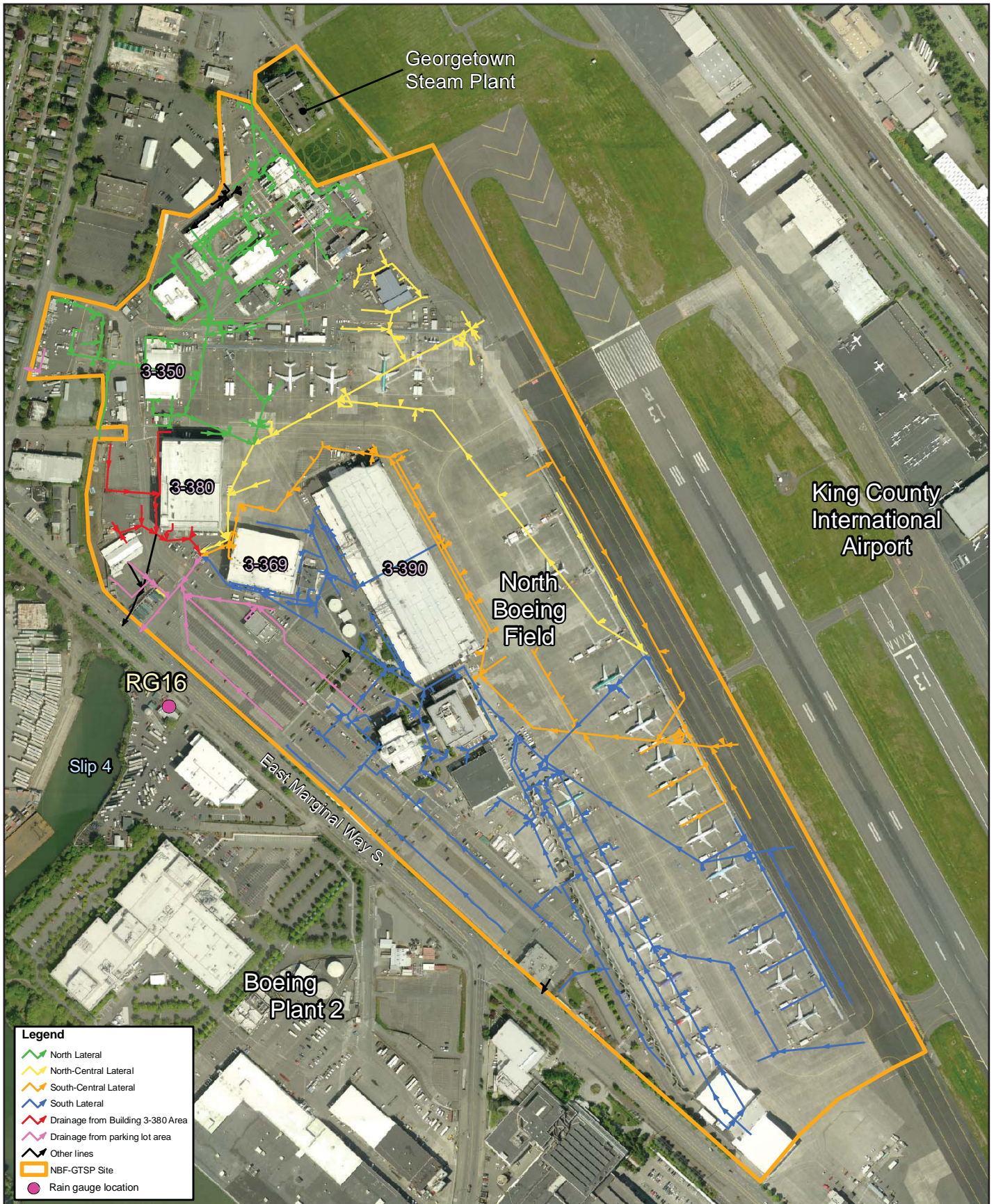
Figure 2. NBF Storm Drain Lines
