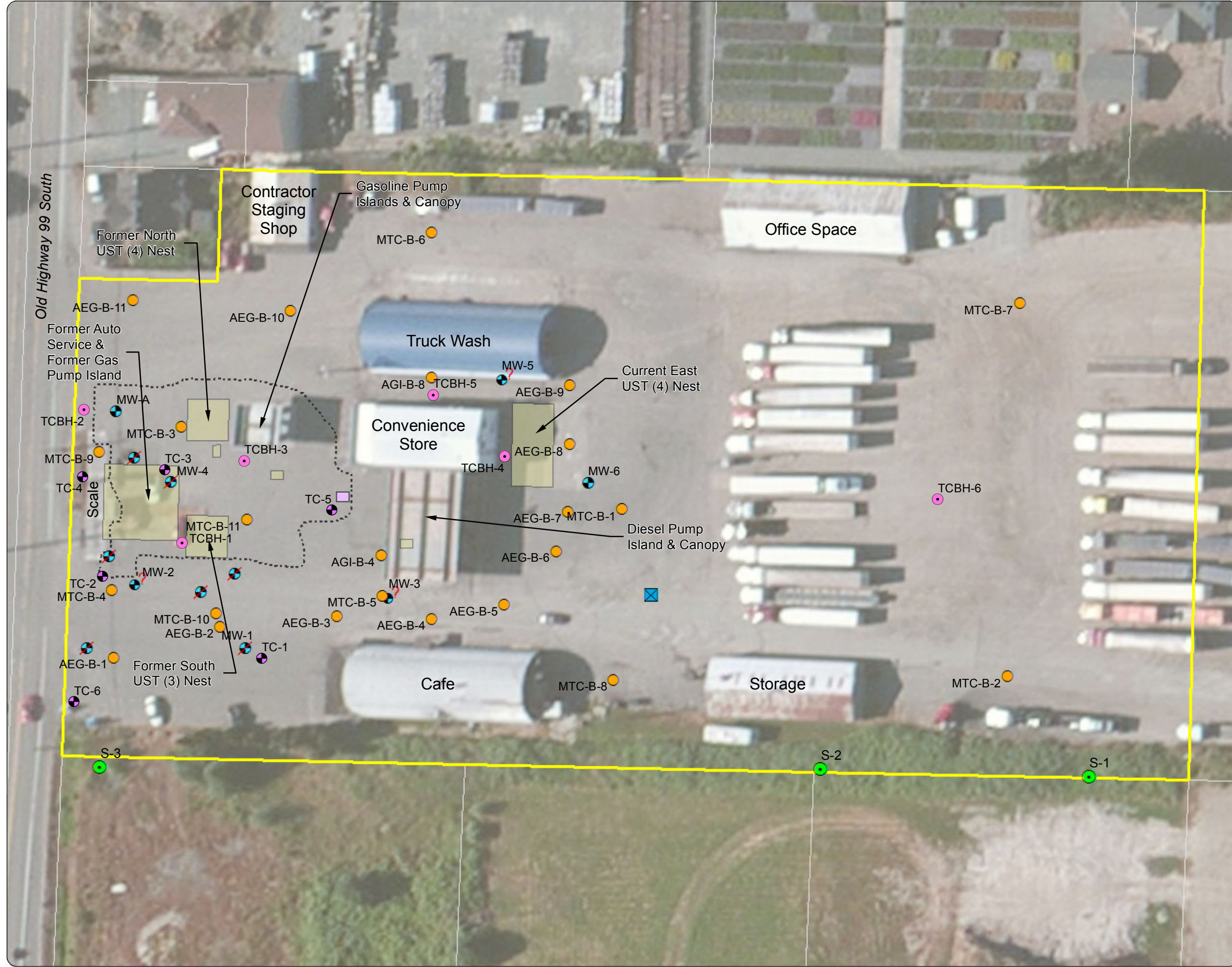
Figure 3 Proposed Subsurface Investigation - Truck City Parcel Truck City Site Mount Vernon, Washington
