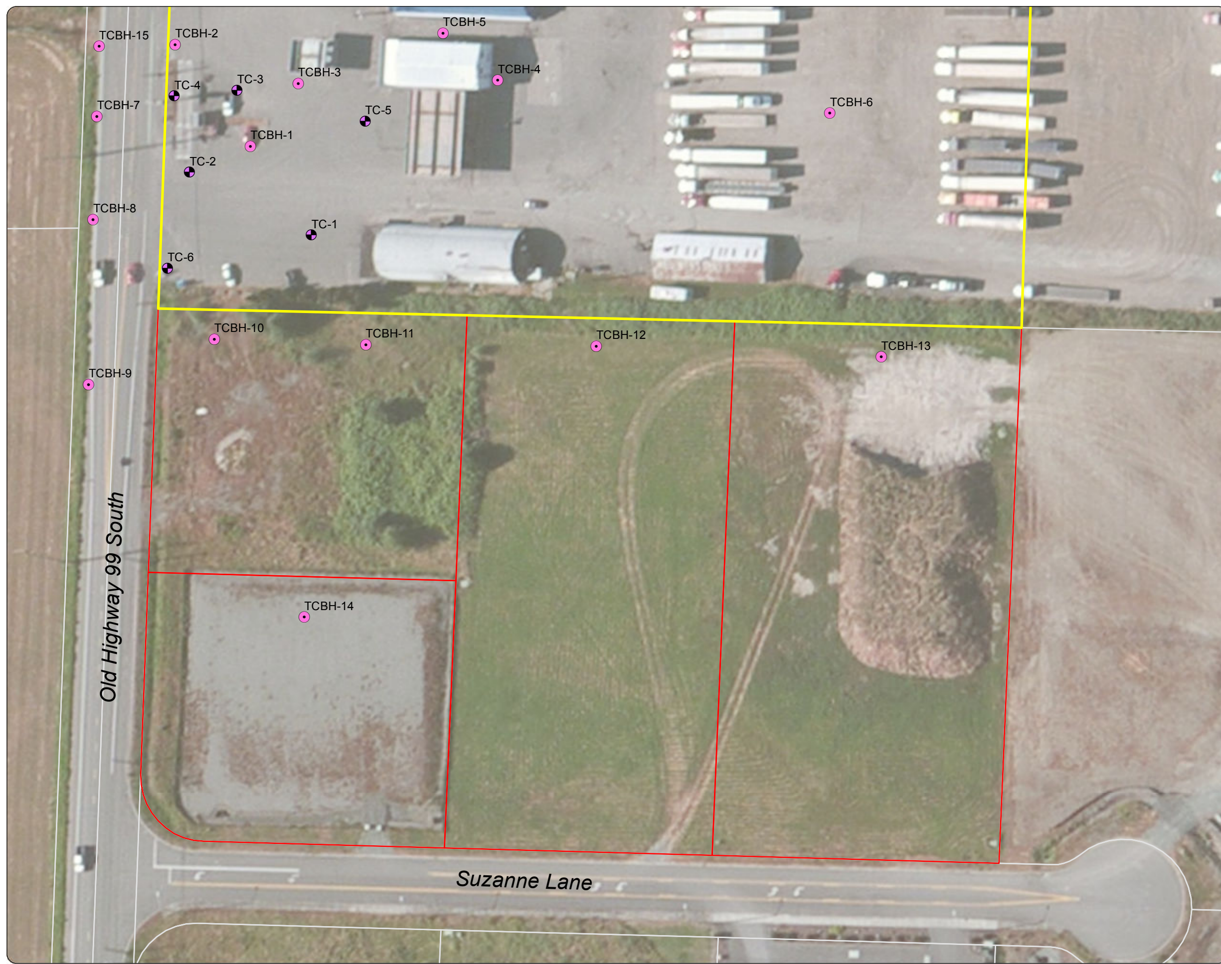
Figure 4 Proposed Subsurface Investigation - Offsite and Southern Parcels
