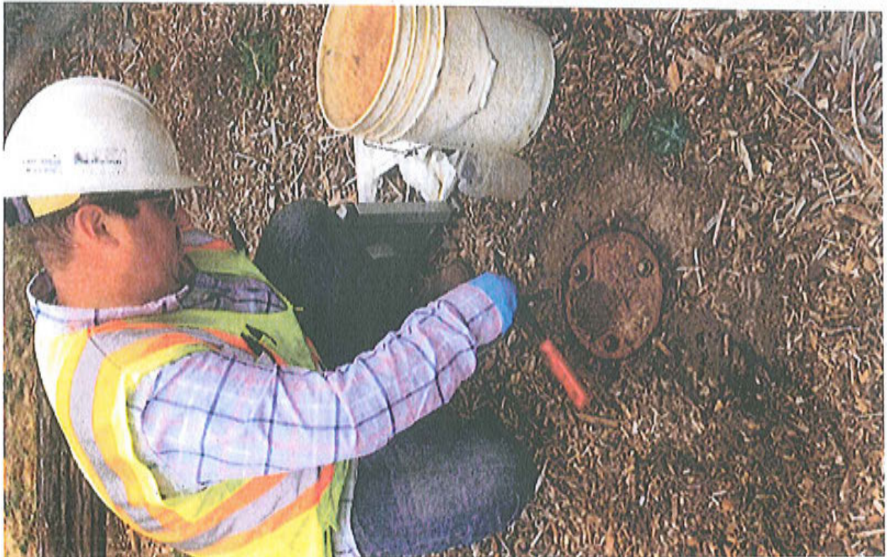
Figure 16. Arcadis-US consultant opening monitoring well monument for groundwater compliance sampling and water elevation measurement at Metro Lake Union Site at public right-of-way MW-22.
