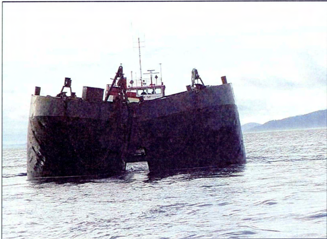
20. Bottom dump barge after unloading at marine habitat bench.
