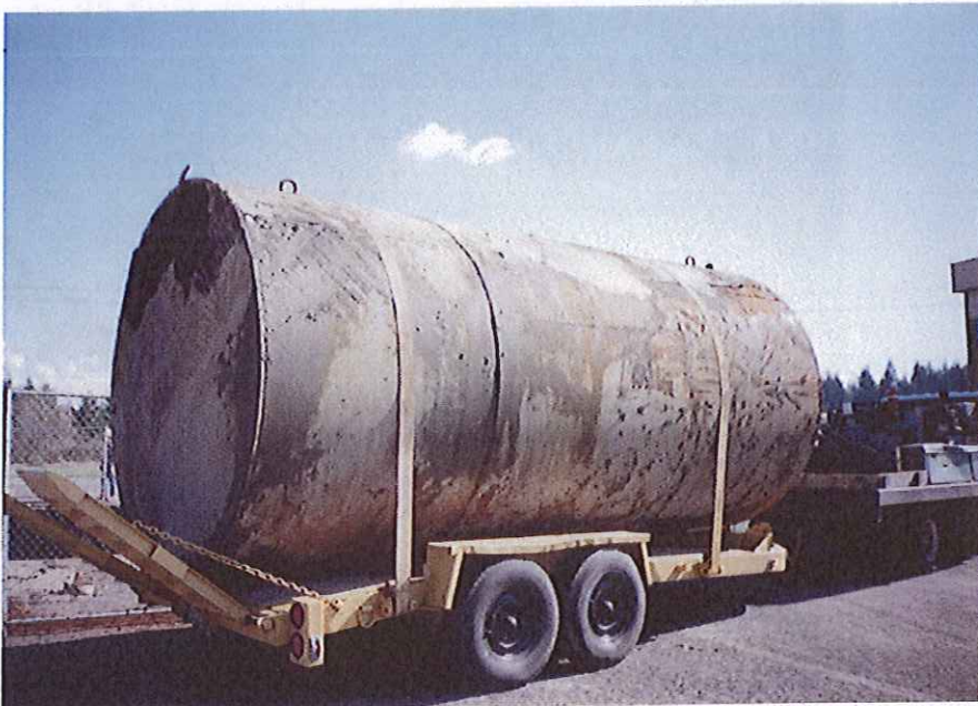
Photo 6 - View of tank T3 after excavation. Tank was in good condition with no holes or pitting, and only minor rust (02/23/96).
