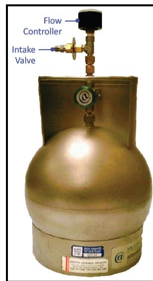
Figure 5: 6-liter Summa canister
