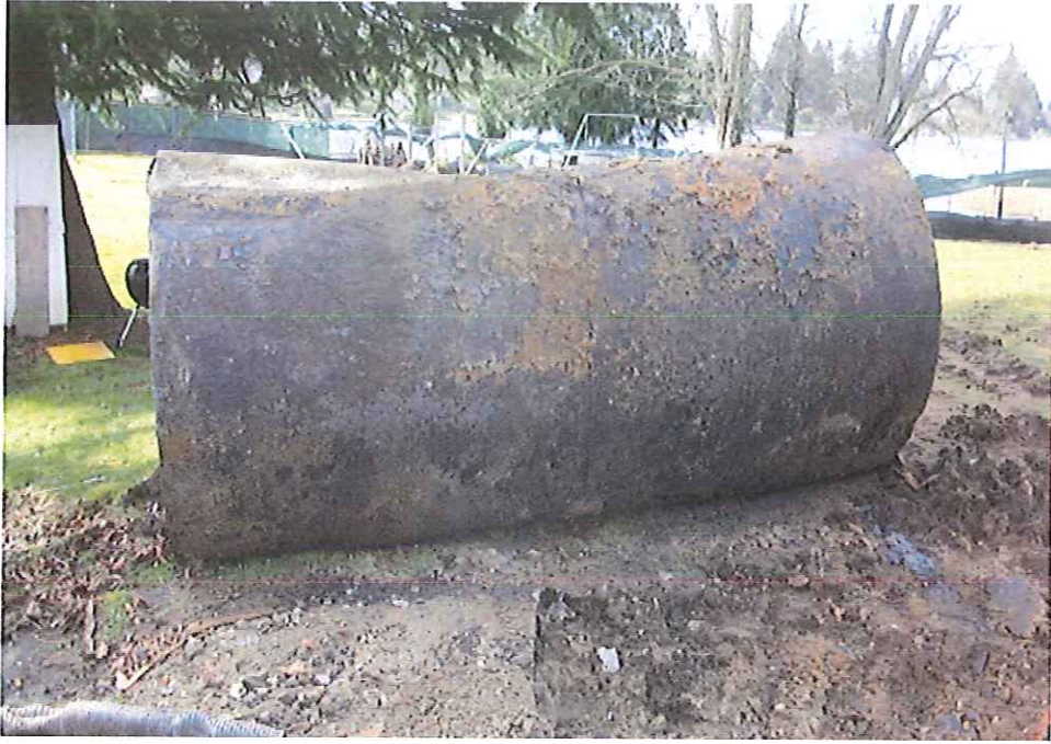
The removed Holly building tank was sized at 60" x 144", with a nominal capacity of 1,780 gallons (40 bbl).
