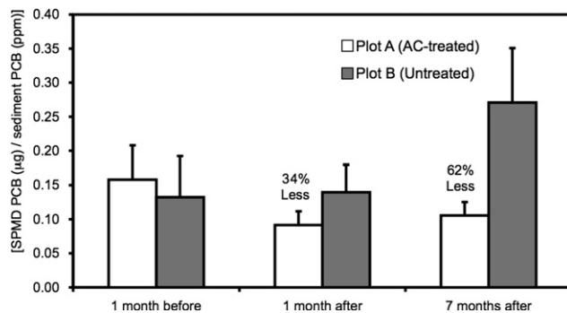
Fig. 5. Comparison of PCB uptakes into SPMD normalized by sediment PCB concentration exposed to the AC-treated Plot A and the untreated Plot B sediment for 28 days. Each column and error bar represents the mean and one standard deviation ( $n = 3\text{--}5$ ).
