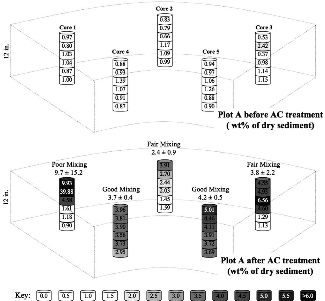
Fig. 4. Comparison of TOC values from sediment cores taken before and after AC treatment in Plot A.
