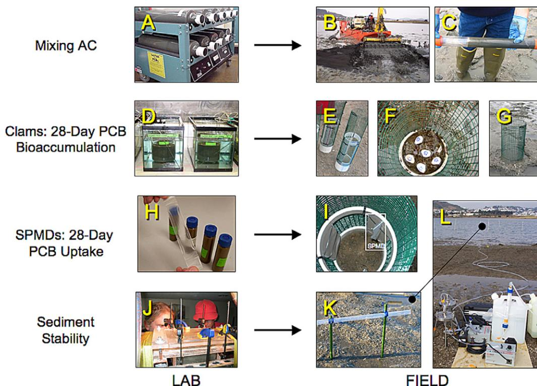
Fig. 3. Comparisons of laboratory and field techniques for assessing (A)–(C) AC mixing, (D)–(G) PCB bioaccumulation in clams, (H)–(I) PCB uptake in SPMDs, and (J)–(L) stability of AC-treated sediment.
