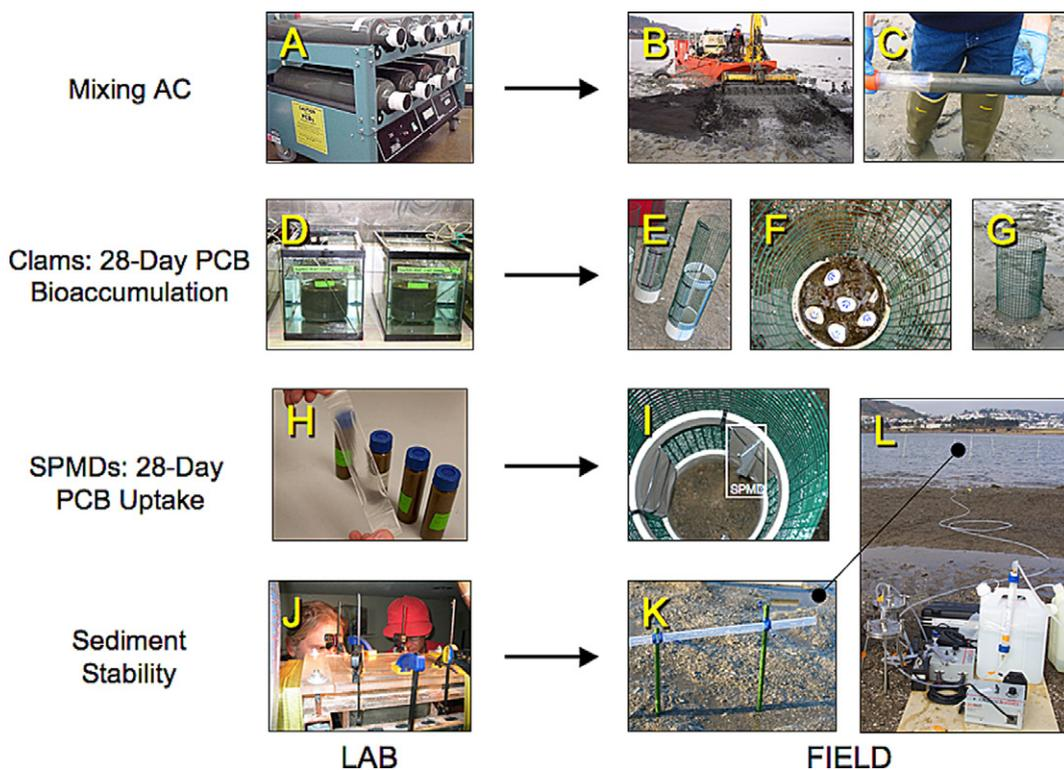
Fig. 3. Comparisons of laboratory and field techniques for assessing (A)–(C) AC mixing, (D)–(G) PCB bioaccumulation in clams, (H)–(I) PCB uptake in SPMDs, and (J)–(L) stability of AC-treated sediment.
