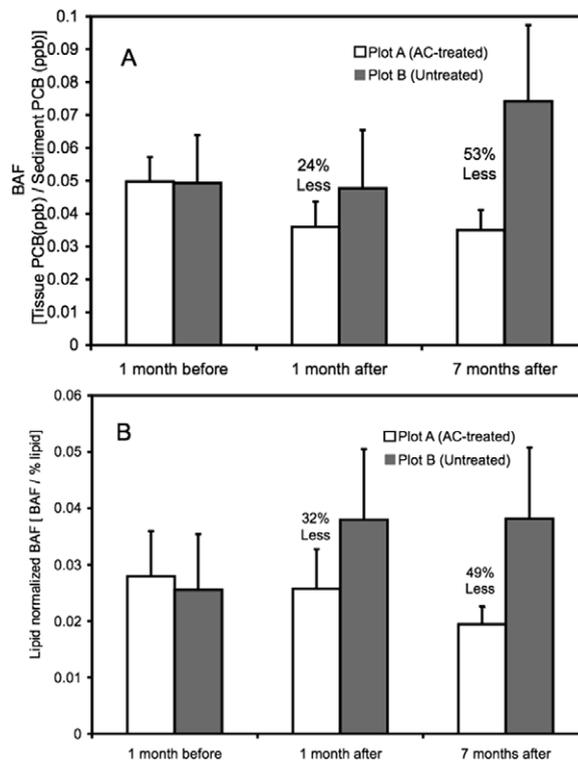
Fig. 6. Comparison of bioaccumulation for field-deployed *M. nasuta* for 28 days. (a) Bioaccumulation factors (BAF = tissue PCB concentration/sediment PCB concentration) and (b) lipid-normalized BAFs for *M. nasuta* exposed to the AC-treated Plot A and the untreated Plot B sediment. PCB tissue concentrations are based on wet weight. Each column and error bar represents the mean and one standard deviation ( $n = 3-5$ ).
