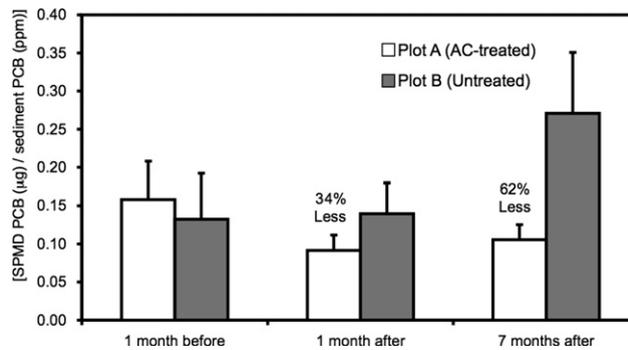
Fig. 5. Comparison of PCB uptakes into SPMD normalized by sediment PCB concentration exposed to the AC-treated Plot A and the untreated Plot B sediment for 28 days. Each column and error bar represents the mean and one standard deviation ( $n = 3-5$ ).
