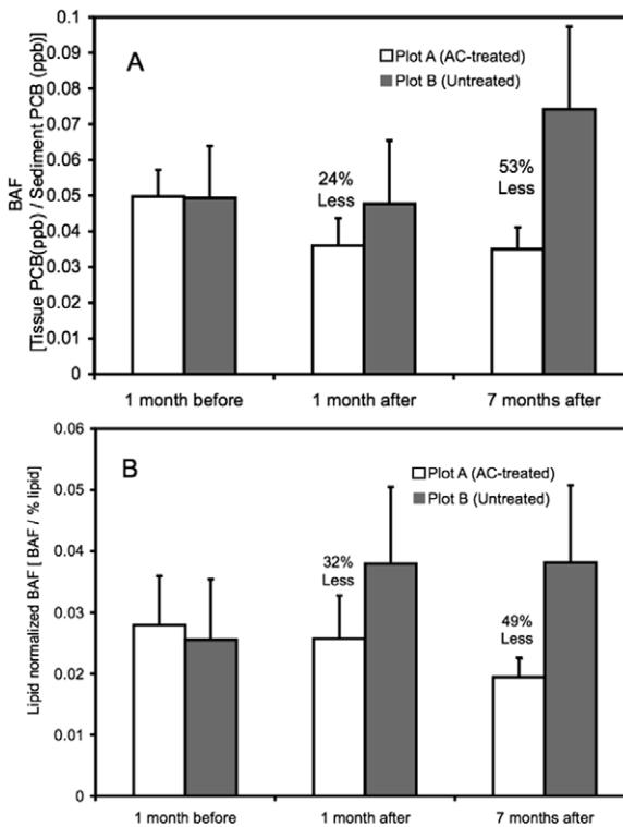
Fig. 6. Comparison of bioaccumulation for field-deployed *M. nasuta* for 28 days. (a) Bioaccumulation factors (BAF = tissue PCB concentration/sediment PCB concentration) and (b) lipid-normalized BAFs for *M. nasuta* exposed to the AC-treated Plot A and the untreated Plot B sediment. PCB tissue concentrations are based on wet weight. Each column and error bar represents the mean and one standard deviation ( $n = 3\text{--}5$ ).
