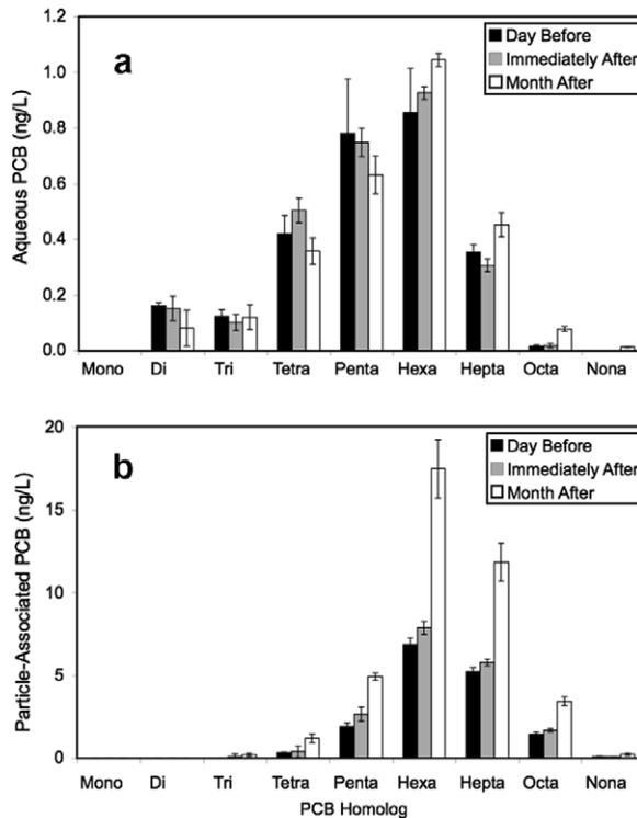
Fig. 8. Comparison of (a) aqueous PCB concentration and (b) particle-associated PCB concentration sampled above Plot A during high tide one day before, immediately after, and one month after AC treatment. Each column and error bar represents the mean and one standard deviation ( $n = 2$ ).
