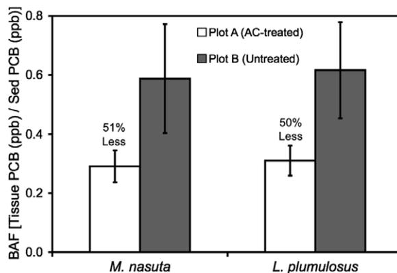
Fig. 7. Comparison of bioaccumulation factors for *M. nasuta* clams and *L. plumulosus* amphipods exposed to the AC-treated Plot A and the untreated Plot B sediment for 28 days in laboratory tests with field cores collected one year after treatment. PCB concentrations in *M. nasuta* tissue are based on dry weight; *L. plumulosus*, wet weight. Each column and error bar represents the mean and one standard deviation ( $n = 4$ ).
