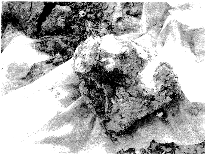
SOLIDIFIED PAINT DEBRIS INSIDE BARREL
