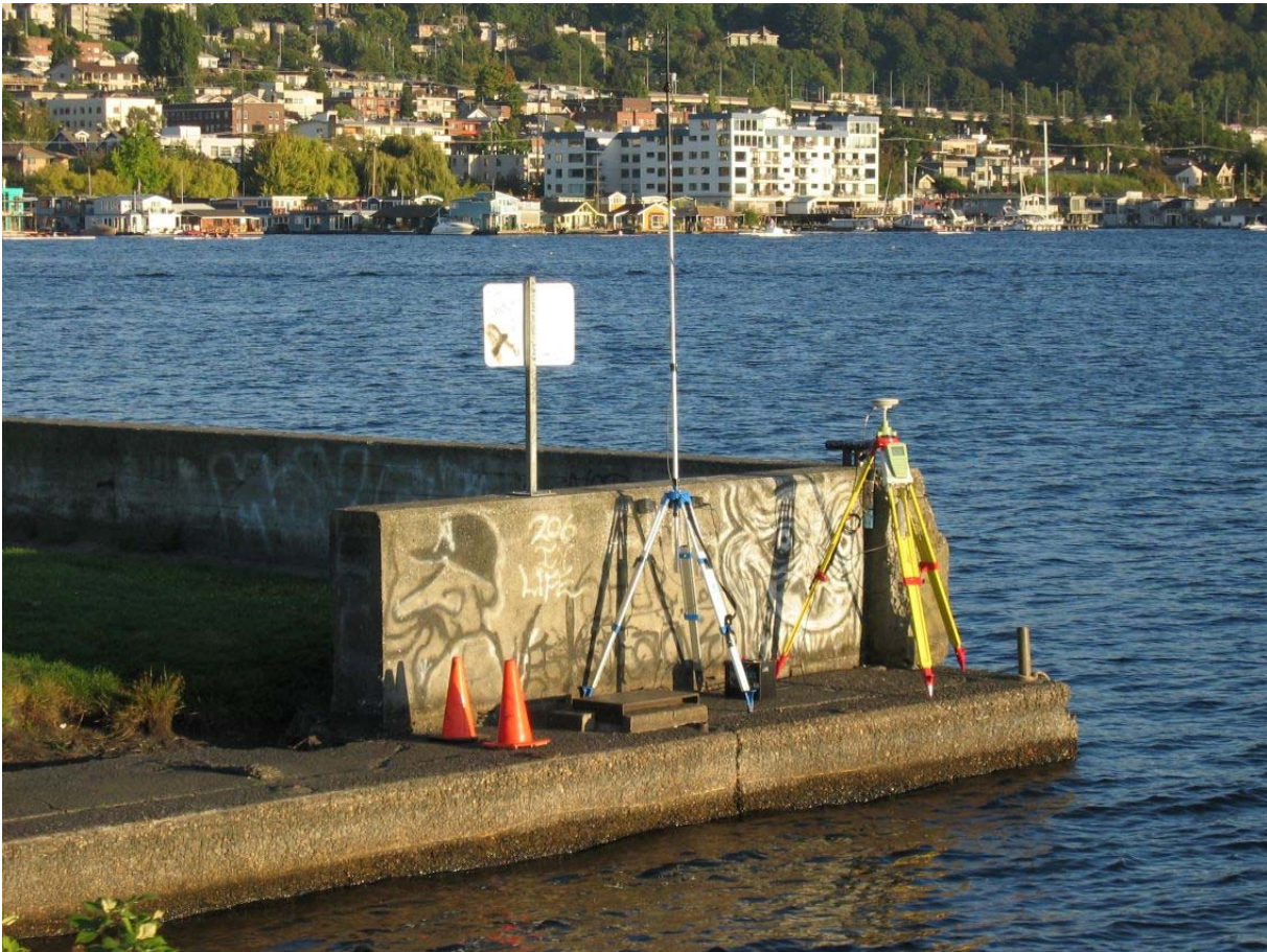
Figure 3-1 - RTK GPS Base Station – Gas Works Park (SAG SY4165)
