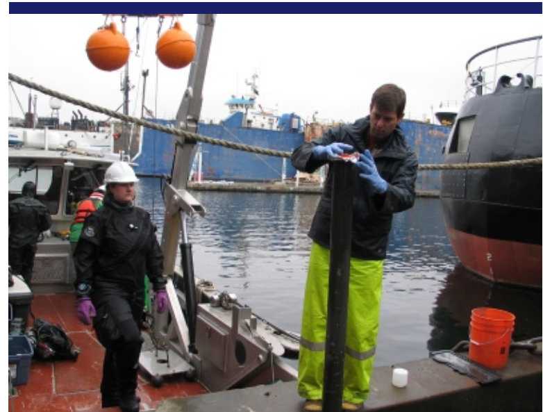
Photo 7 Herrera and RSS personnel capping NS16 core tube.
