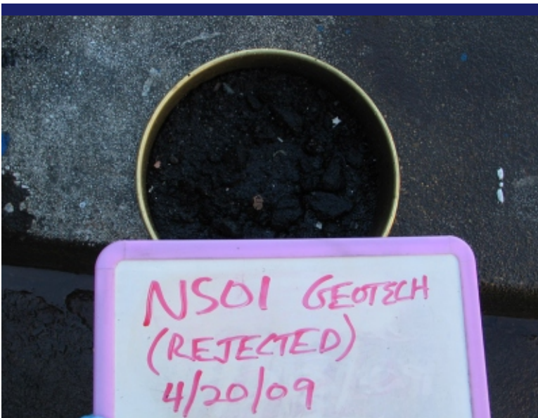
Photo 16 NS01-G core sieved fraction with sandblast (loose and chunks) and paint chips.
