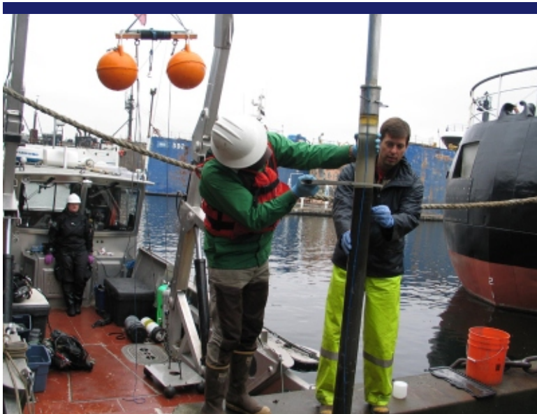
Photo 6 Herrera and RSS personnel cutting NS16 core tube.
