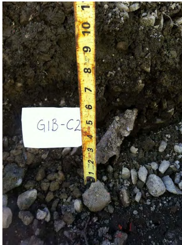
Photograph 6. Potential Sandblast Grit at G1B-C2 Sample Location.
