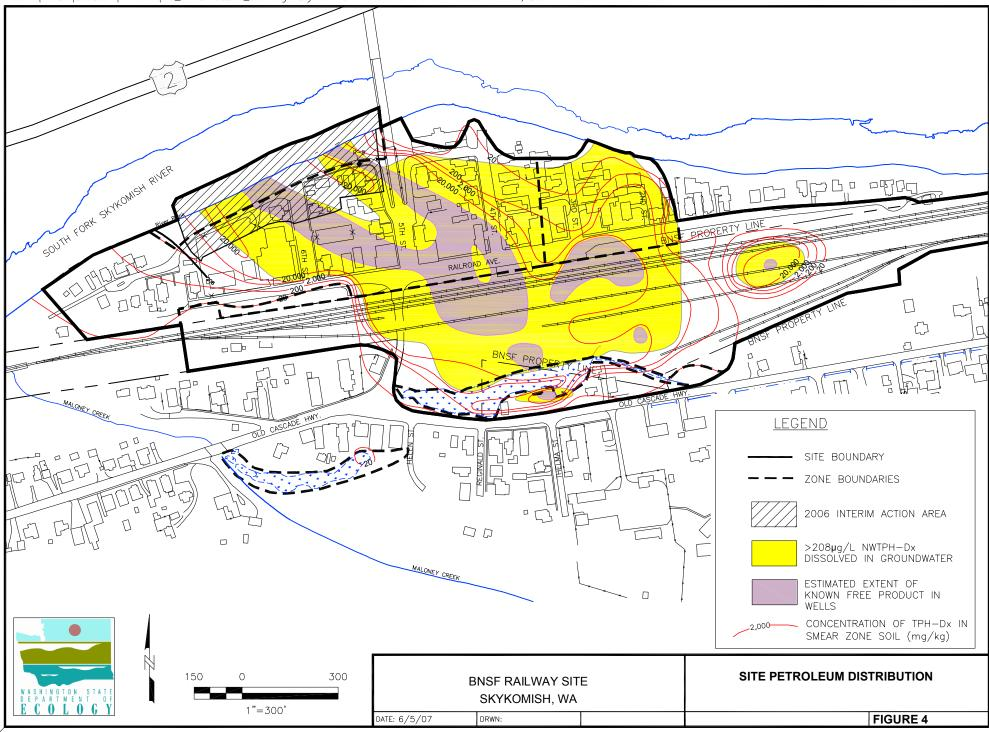
File: P:\CADD\BNSF-Skykomish\ECOLOGY\10-11-07\FIG\_5-SITE\_ZONES.dwg Layout: FIG 5 User: emarshall Plotted: Oct 16, 2007 - 10:07am Xref's:
