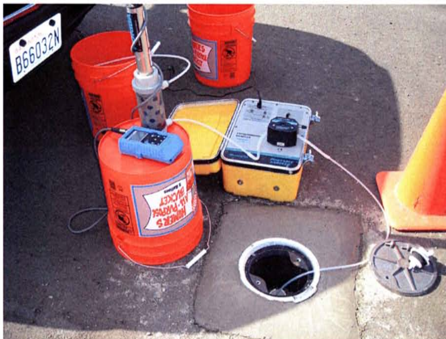
Photograph No. 7: View of well development equipment setup on MW-02.
