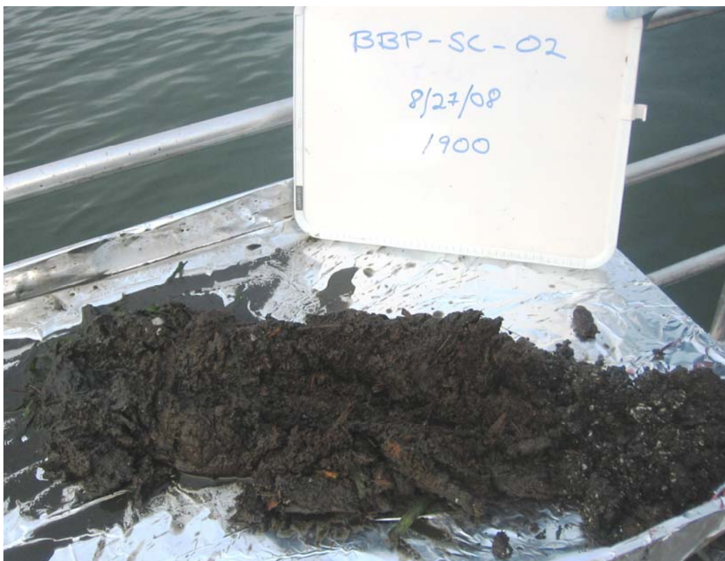
Photograph 10 - Sediment core sample BBP-SC-02, 0 to 3 feet. Slightly gravelly, silty SAND (SM) with abundant wood debris (wood chips, sticks, and bark).
