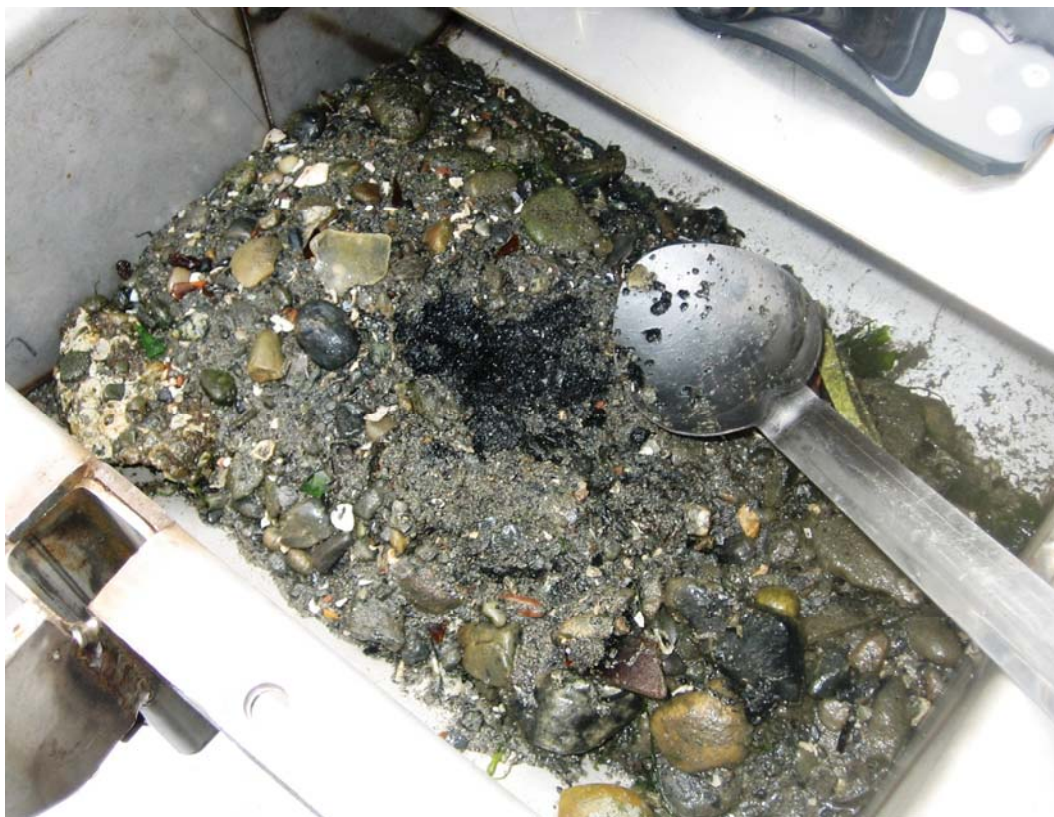
Photograph 1 - Surface sediment grab sample RGH-SS-02. Silty, sandy GRAVEL (GM) with moderate cobbles.
