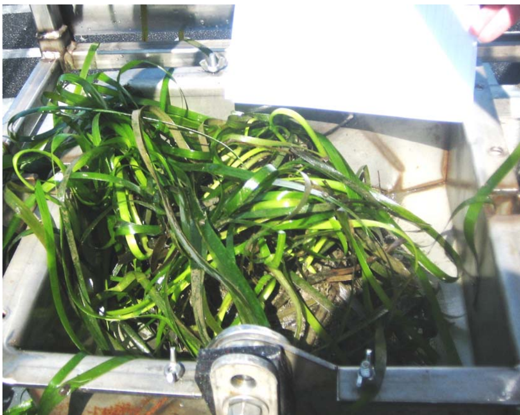
Photograph 8 - Sediment surface grab sample BBP-SS-02. Silty SAND (SM) with scattered gravel and cobbles, moderate shell fragments, and abundant eel grass.
