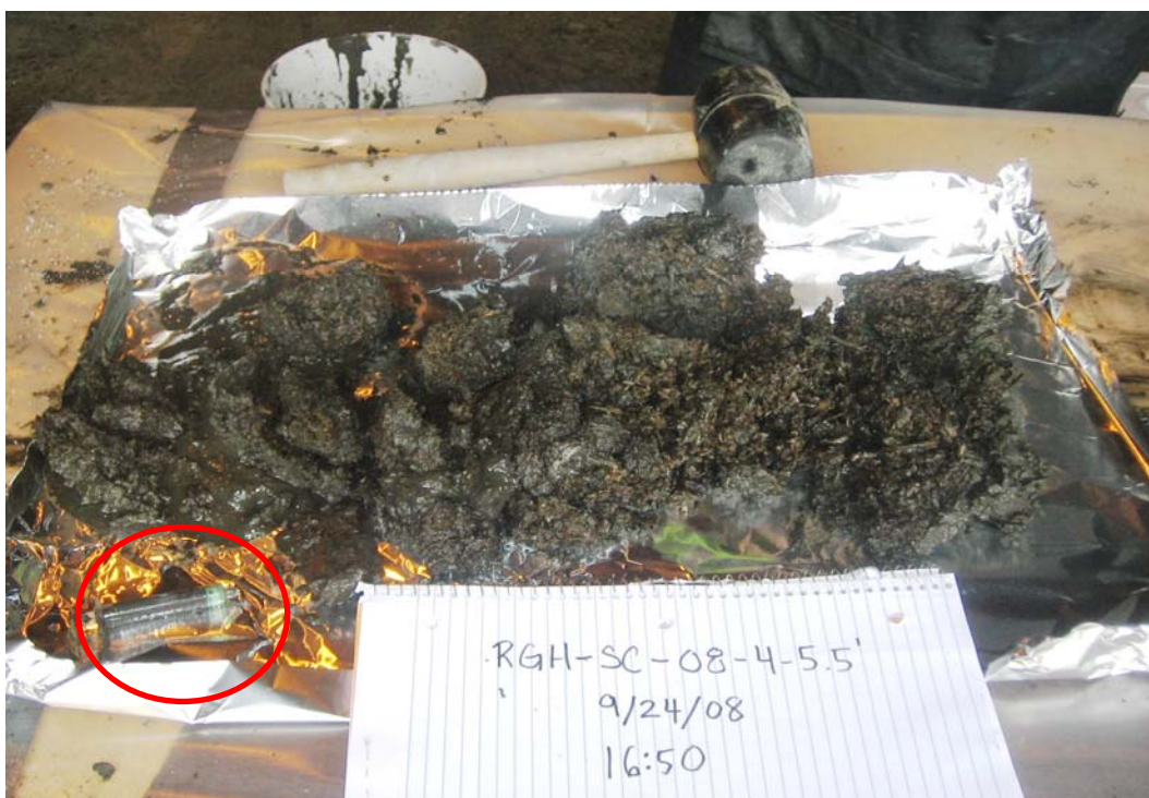
Photograph 7 - Sediment core sample RGH-SC-08, 4 to 5.5 feet. Silty PEAT (PT) with wood pieces (0.5- to 2-inch), with a plastic syringe in shoe (lower left corner of photograph).
