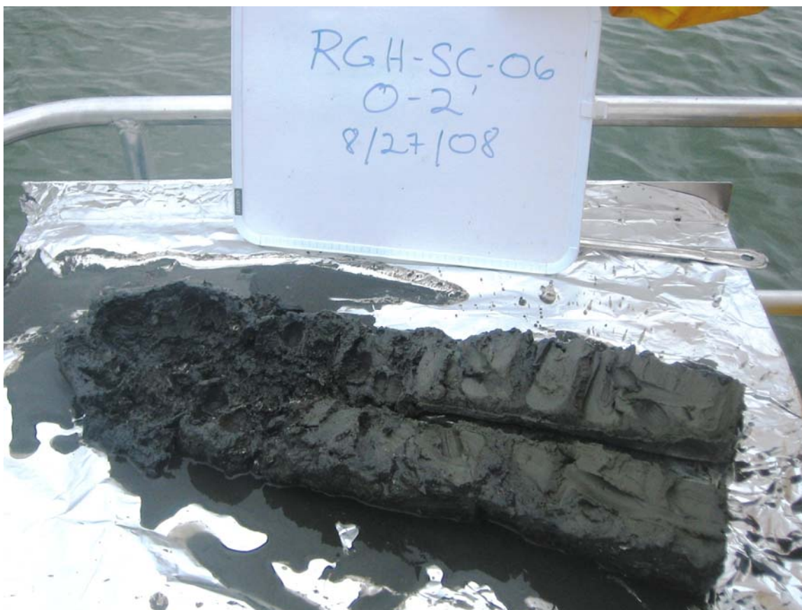
Photograph 2 - Sediment core sample RGH-SC-06, 0 to 2 feet. Sandy SILT to clayey SILT (ML).
