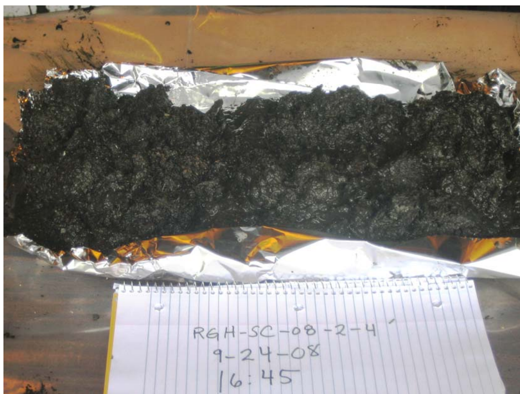
Photograph 6 - Sediment core sample RGH-SC-08, 2 to 4 feet. Sandy SILT (OL) with increased wood chips/sawdust with depth.
