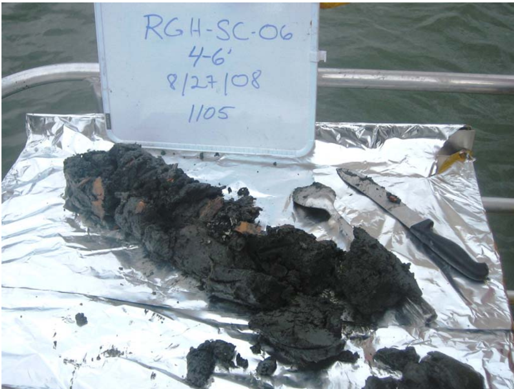
Photograph 4 - Sediment core sample RGH-SC-06, 4 to 6 feet. Layers of wood chips/fragments (1- to 3-cm thick) with shell hash.
