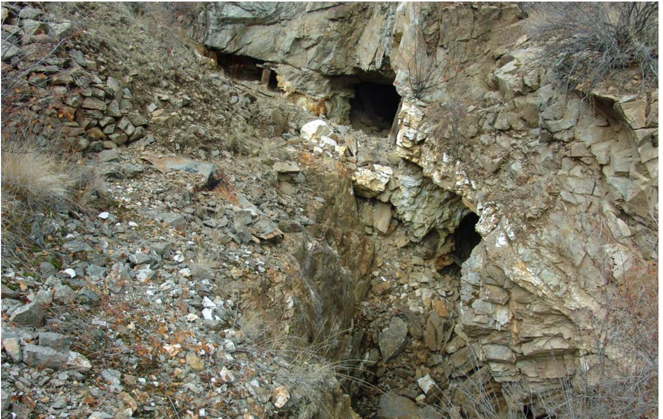
A portion of the surface workings and stopes associated with the Triune Mine.
