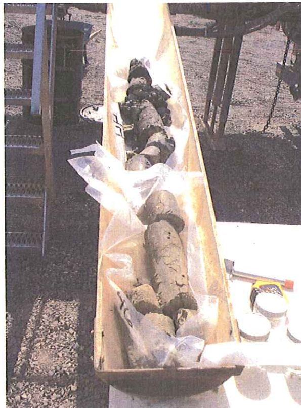
Photo 6: : Photograph of inorganic clay/sandy clay horizon identified at 40 to 45 ft below ground surface.
