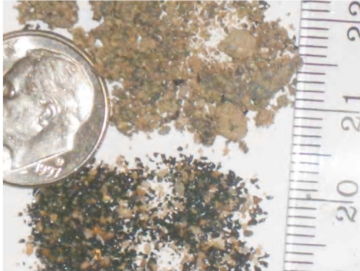
Typical replacement sand is shown above, existing granulated slag is shown in bottom section of top photograph.
