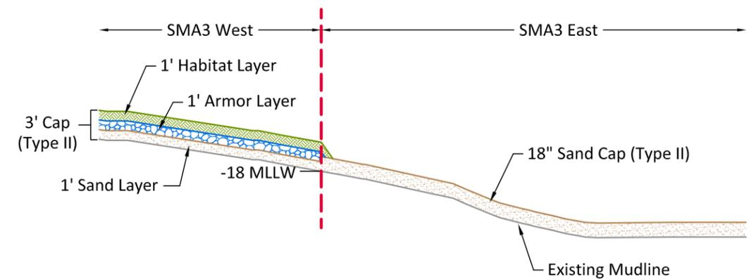
**Cross Section Schematic**
