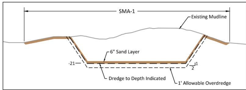
**SMA 1 Cross Section Schematic**
