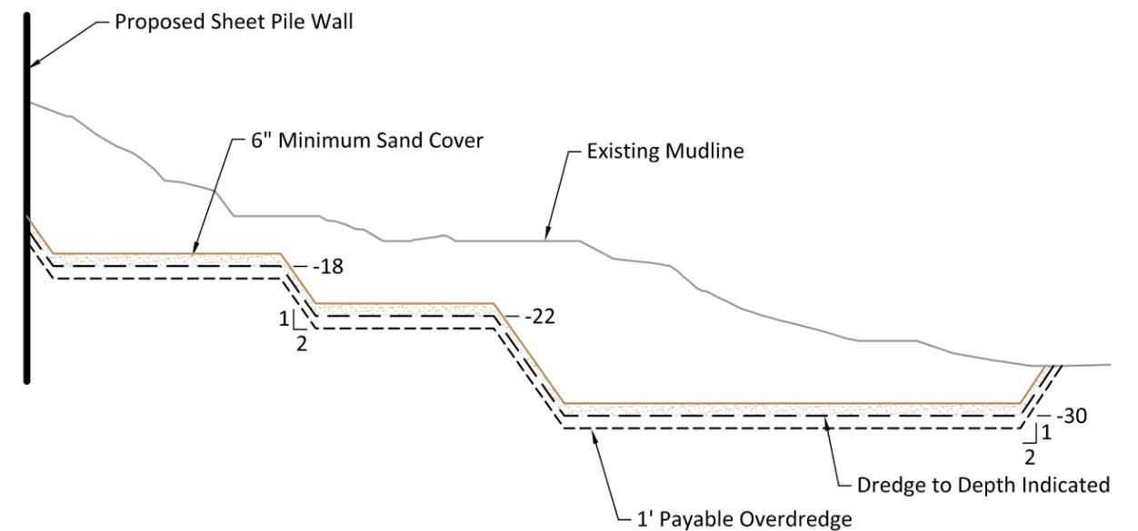
**Cross Section Schematic**
