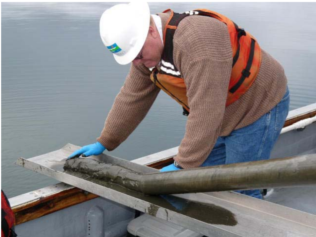
Photograph 2 - Extruding sediment core sample on board as described in the SAP.
