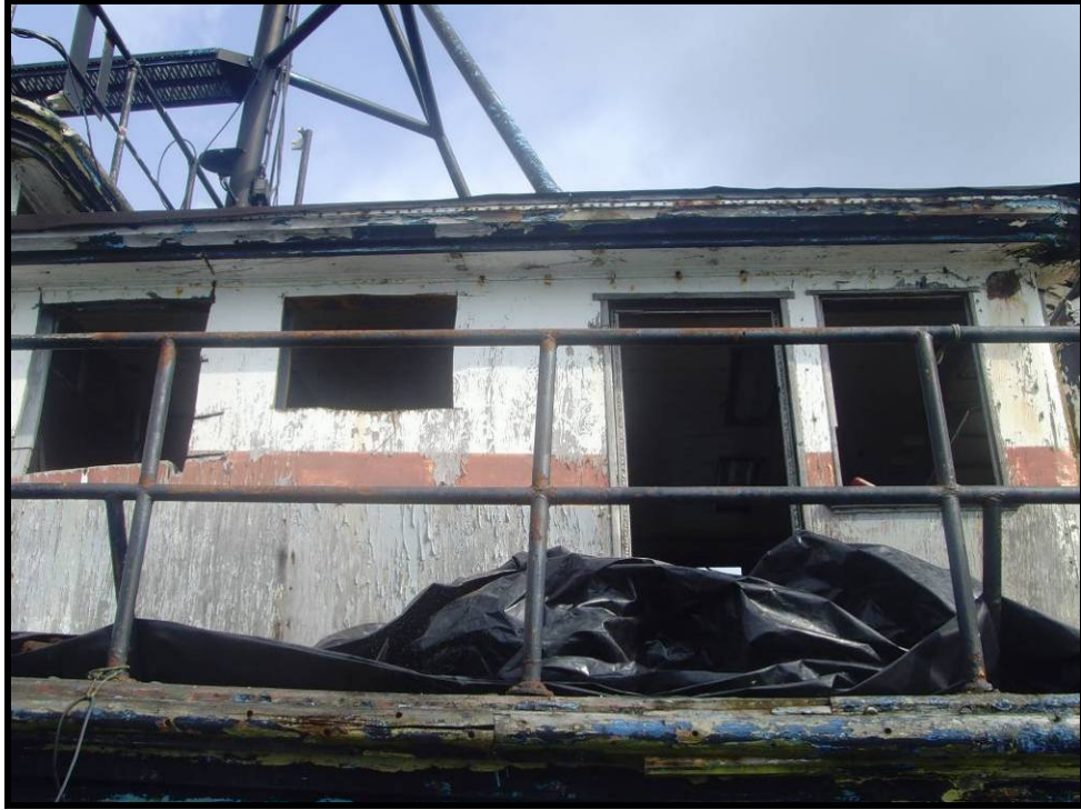
Figure 4. The pilot house on the Enchantress showing cut marks where portholes have been removed (view east).
