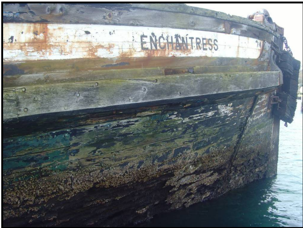
Figure 5. Hull damage from Teredos (view west).
