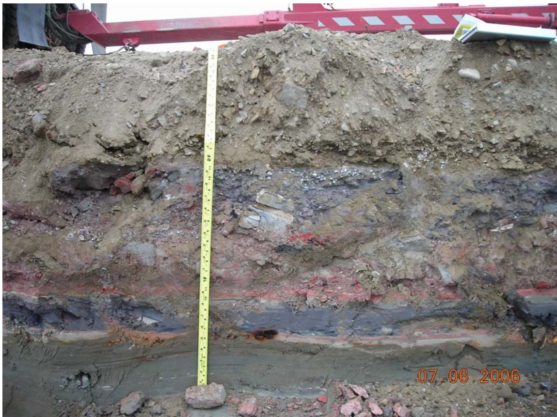
Profile along I-3a and I-2 boundary showing colored concrete-like material.
