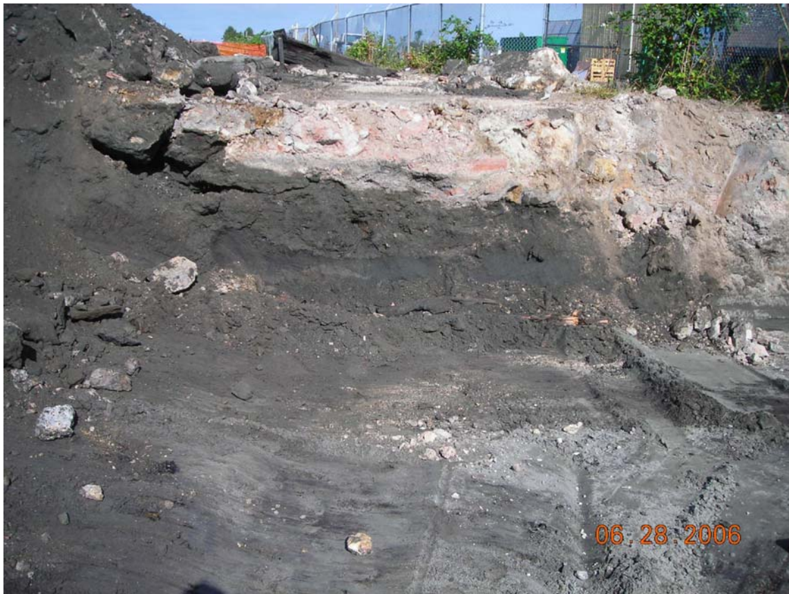
Colored concrete-like material overlying black sand material in I-5, looking west.
