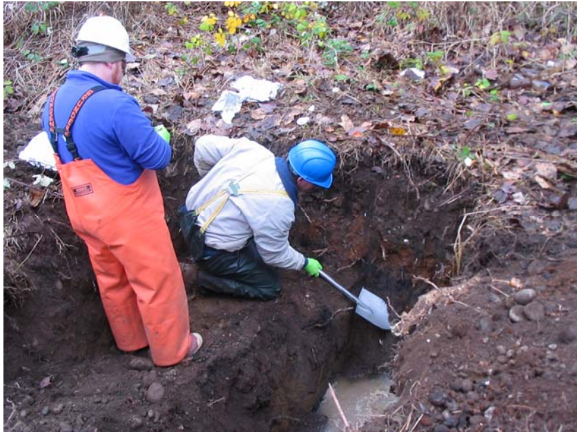
Researchers collect samples and examine layers of soil and contaminants in the old landfill.
