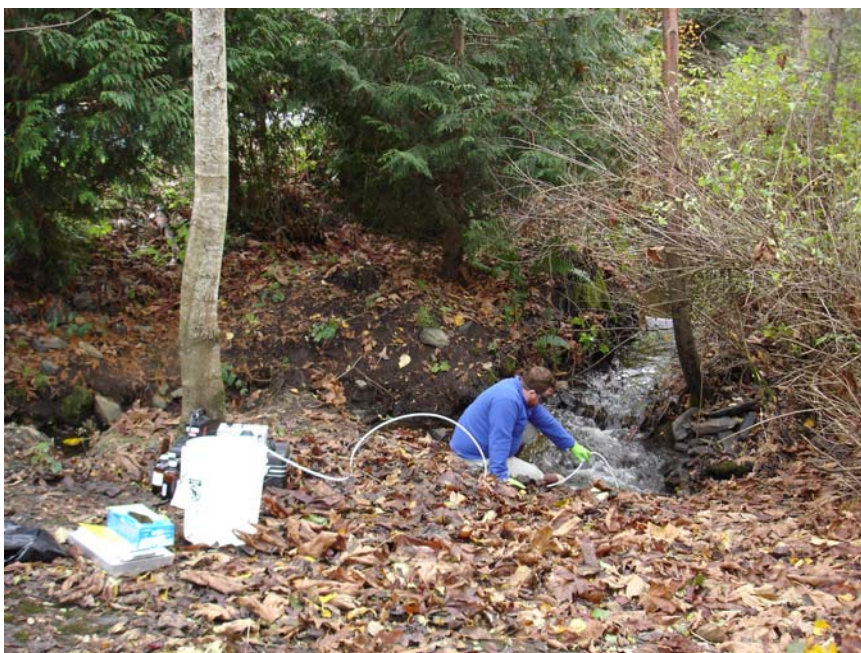
Photo 3. Surface water sample collection using a peristaltic pump. The reference surface water station is shown in the photo.
