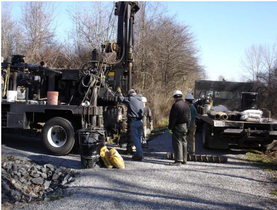
Photo 7. Standard rubber tire hollow-stem auger drill rig used to install monitoring wells. Monitoring well SB-24 is shown in the photo.
