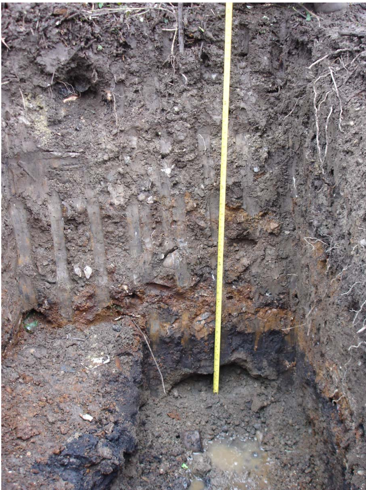
Photo 14. Historical landfill debris underlain by a black organic-rich silt (native) observed at test pit TP-23.
