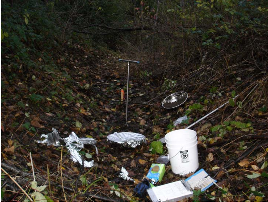
Photo 5. Soil sample collection using a stainless steel hand auger. Station HA-8 is shown in the photo.
