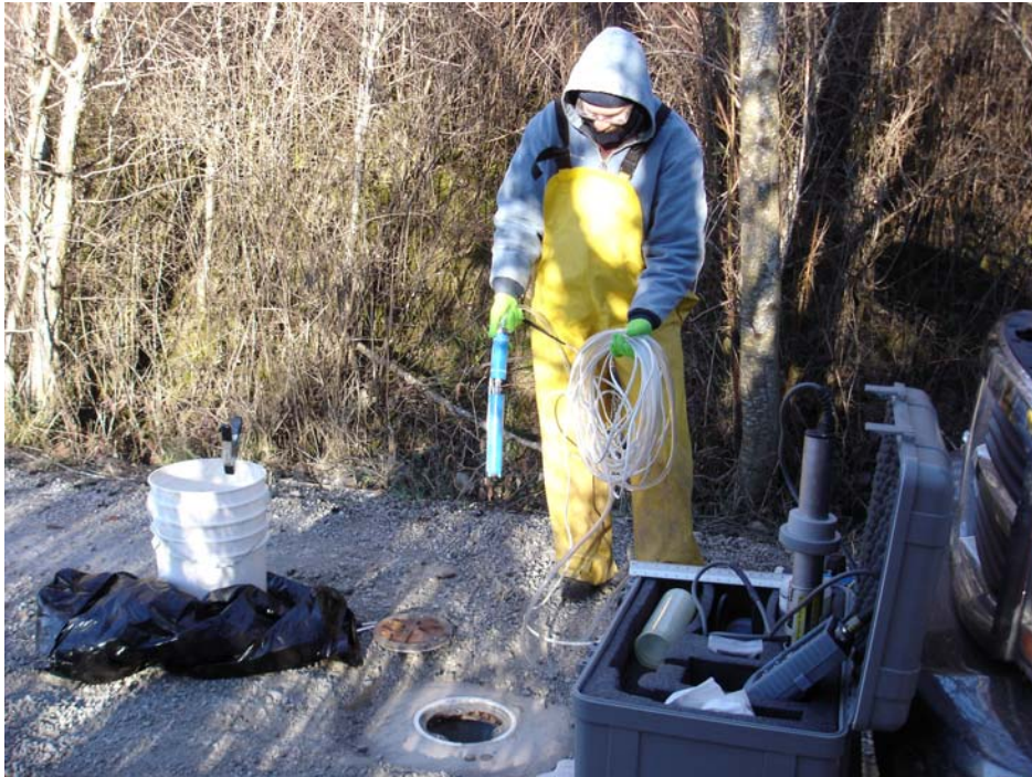
Photo 11. Centrifugal pump used to develop monitoring wells.
