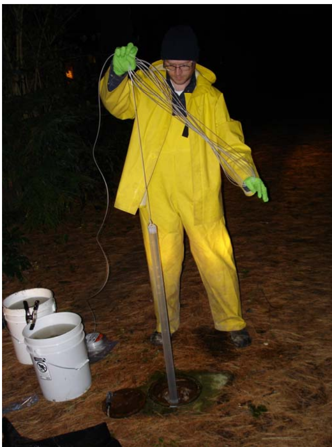
Photo 2. Groundwater purging using a new, disposable Teflon® bailer. Monitoring well MW-6D is shown in the photo.
