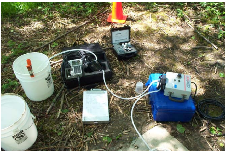
Photo 1. Groundwater purging through a flow-through cell using a peristaltic pump. Piezometer SB-28 is shown in the photo.
