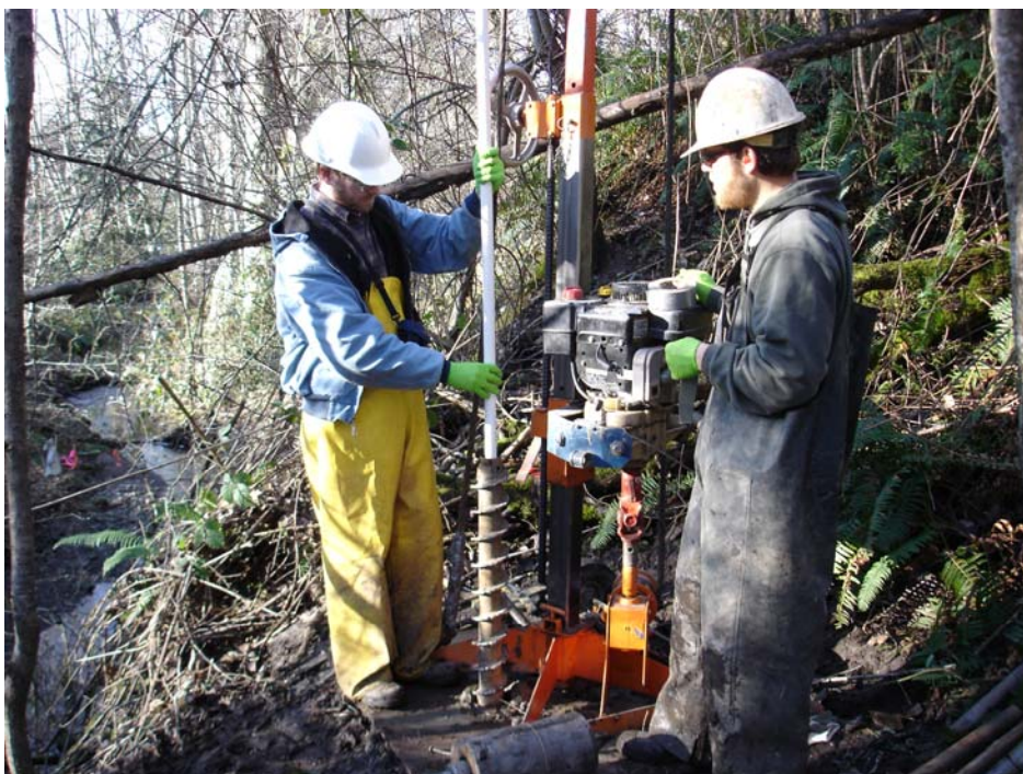
Photo 9. Acker® portable hollow-stem auger drill rig used to advance soil borings and install piezometers. Station SB-14 is shown in the photo.
