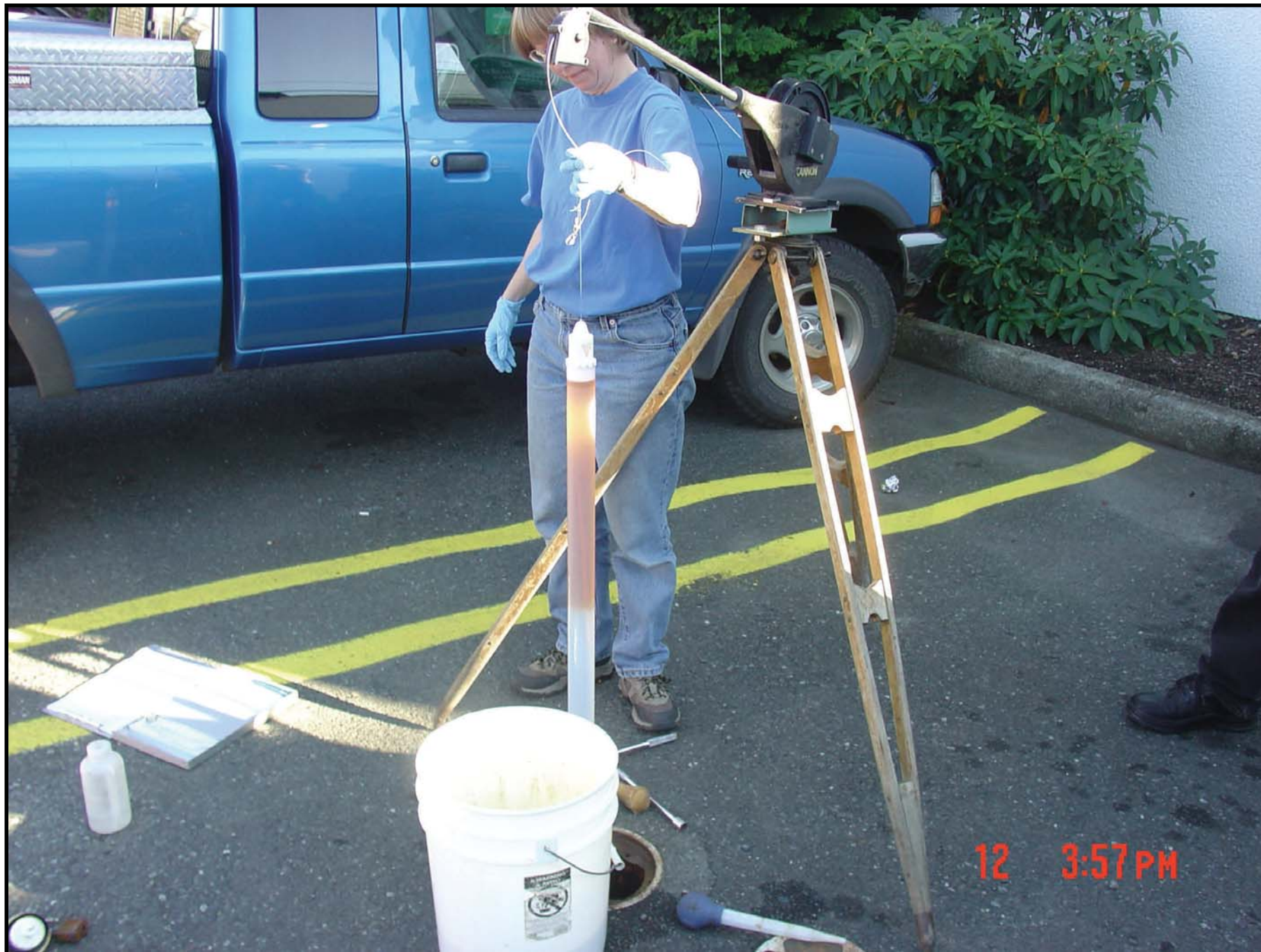
Figure 7. Free product gasoline found on groundwater.
