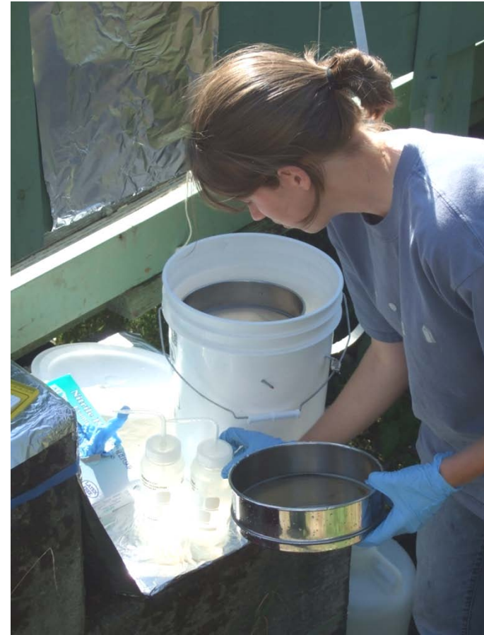
Figure B-7. Rinsing sieves to collect coarser (sand) fraction of suspended sediments.
