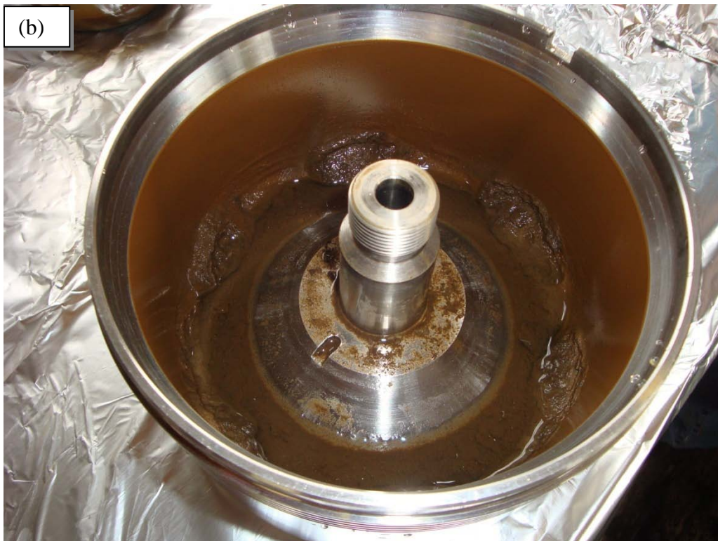
Figure B-5. (a) Removing excess water from centrifuge bowl, and (b) view of the retained suspended sediments.
