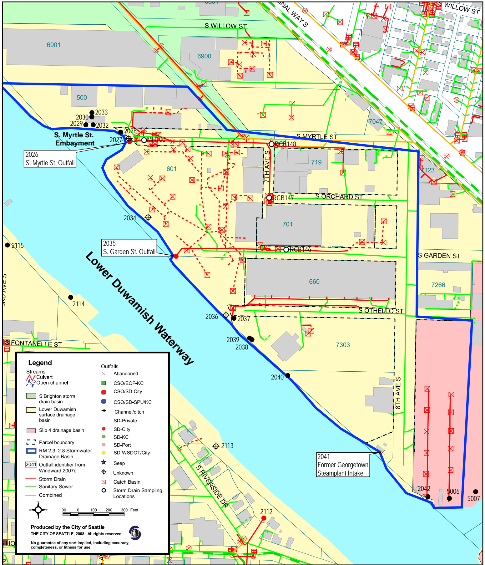
Figure 5. RM 2.3–2.8 East (Seattle Boiler Works to Slip 4) Storm Drain System and Sampling Locations
