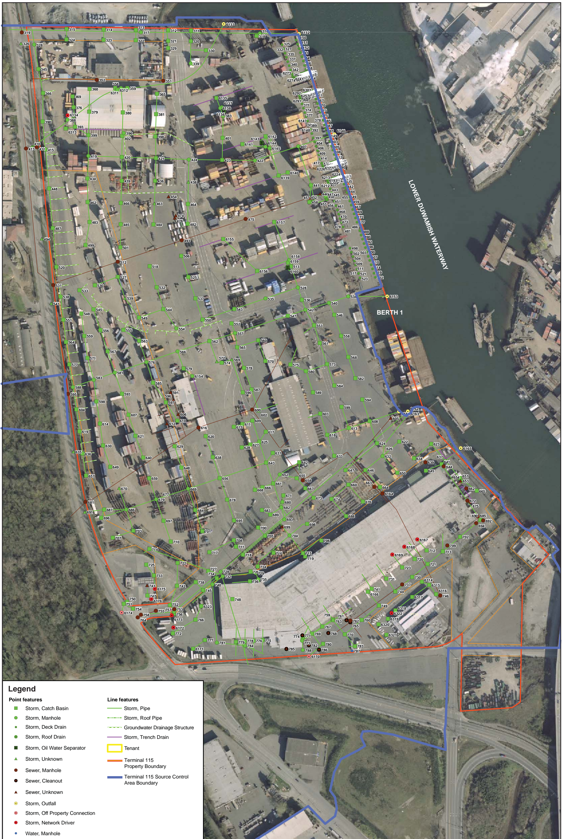
Figure 7b. Storm Drain and Sewer Lines and Structures at Terminal 115
