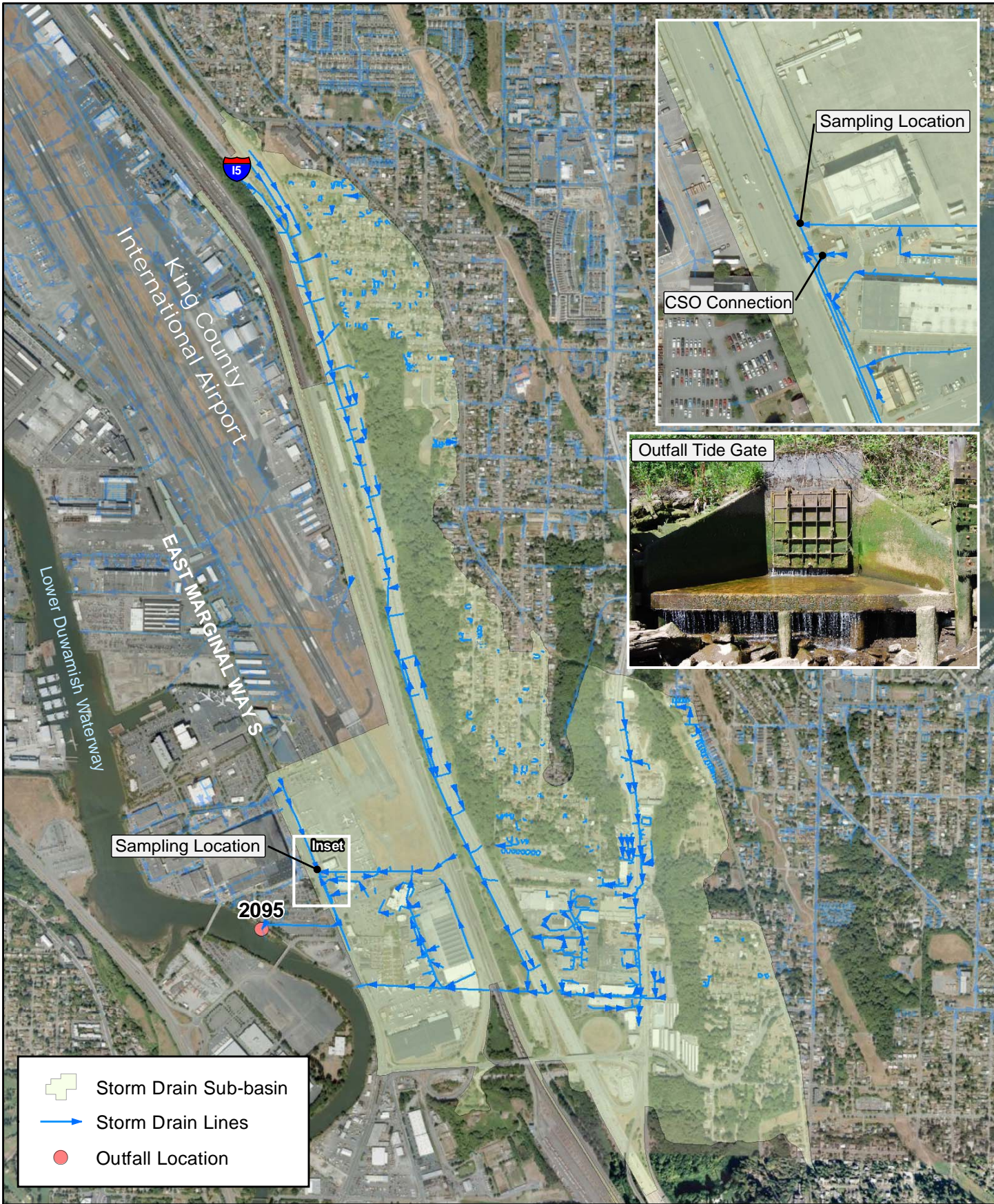
Figure 2. Norfolk Storm Drain Sub-basin and Outfall Location (2095)
