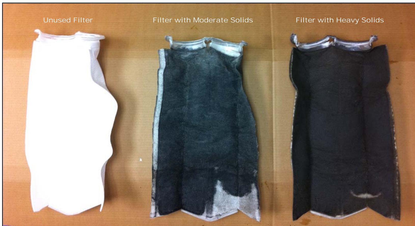
Figure 10. Interior of Filter Bags Used to Collect Filtered Solids
