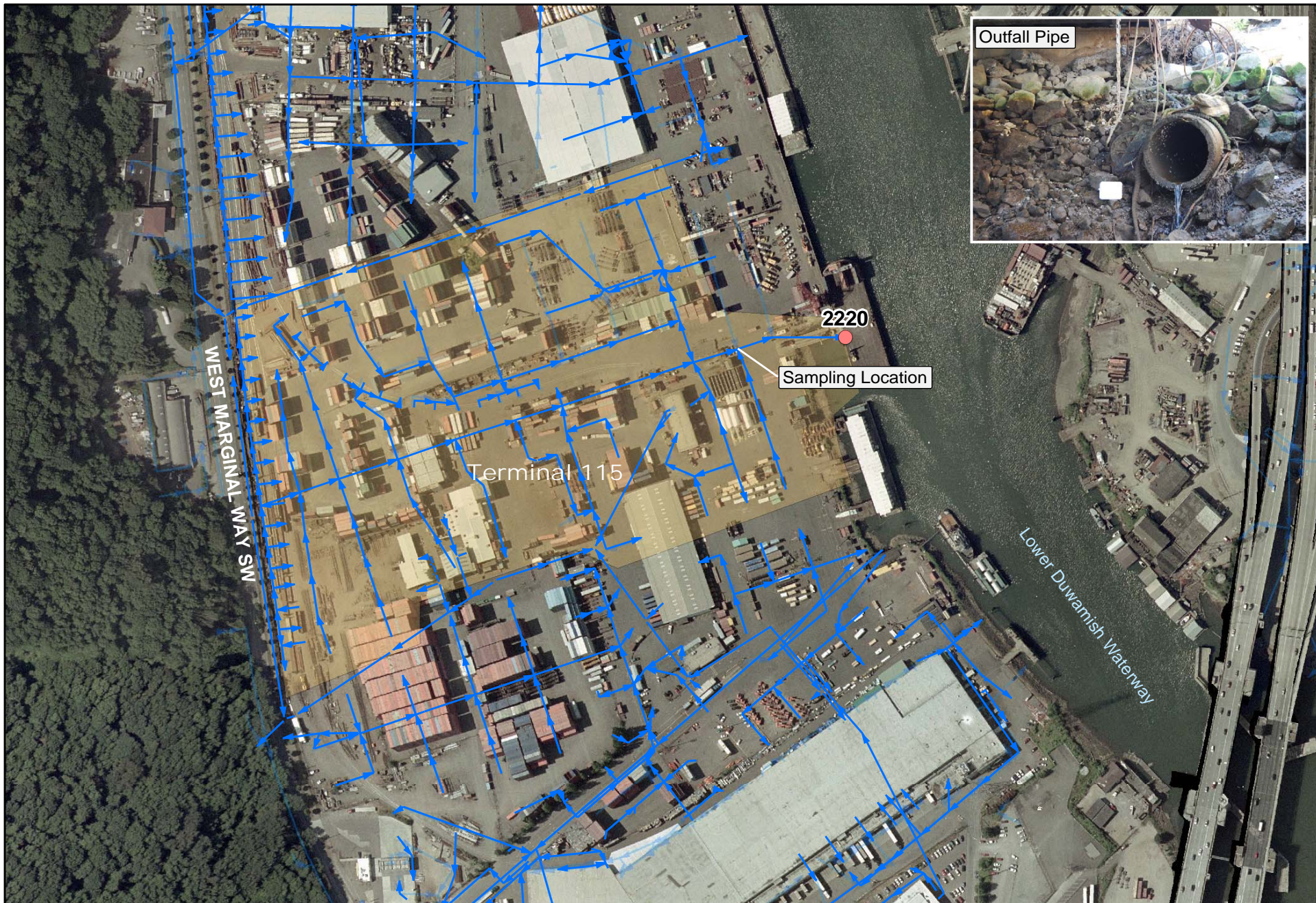
Figure 4. Port of Seattle Terminal 115 Storm Drain Sub-basin and Outfall Location (2220)
