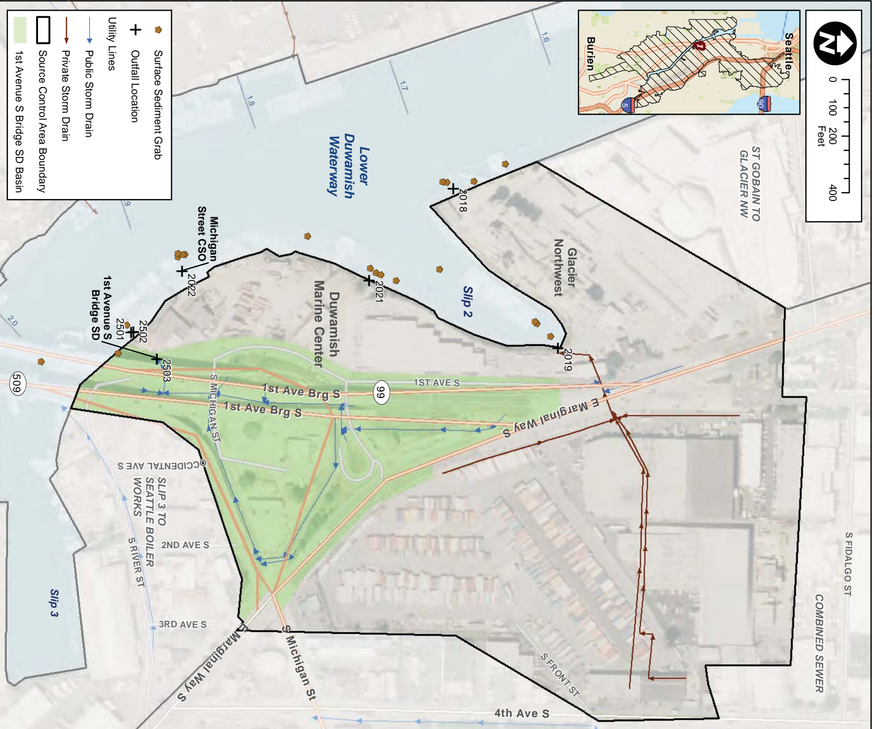
Figure 3-38a. Surface Sediment Sample Locations near RM 1.7-2.0 East (Slip 2 to Slip 3)
