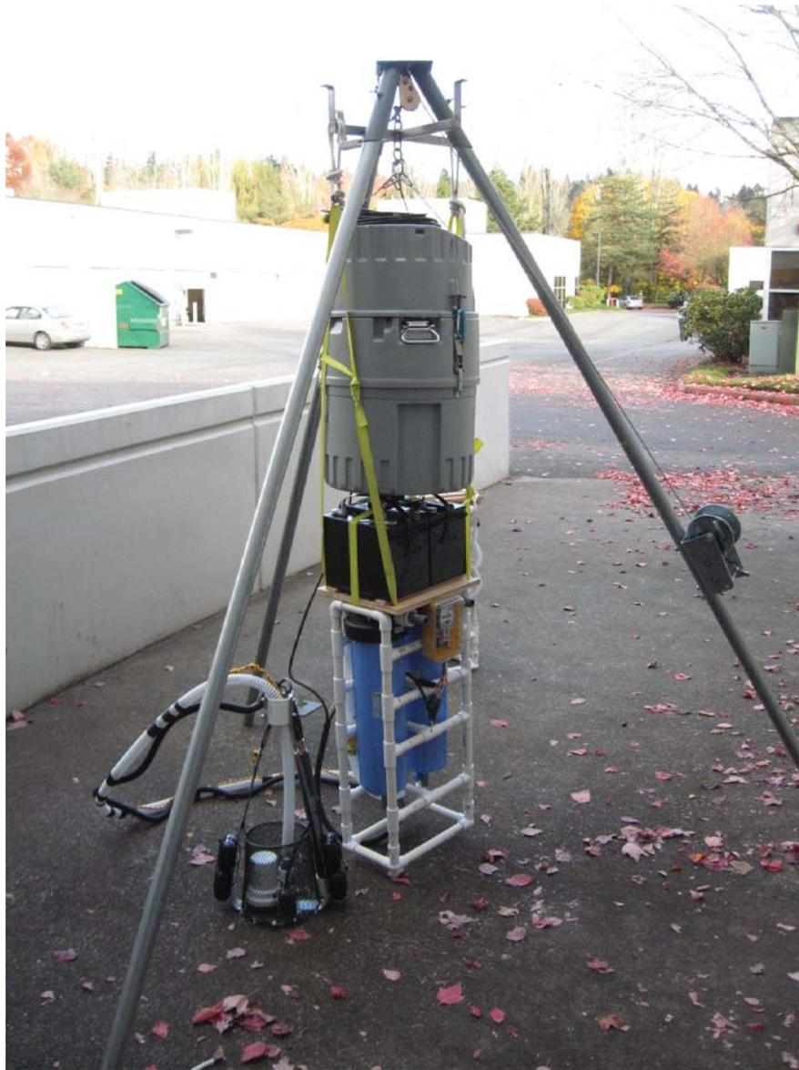
Figure 6. ISCO Whole Water Sampler
