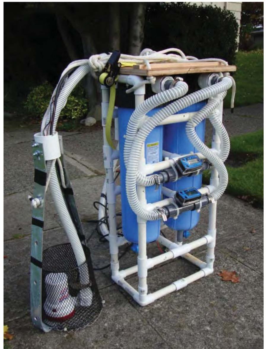
Figure 7. Suspended Solids Filtration Unit
