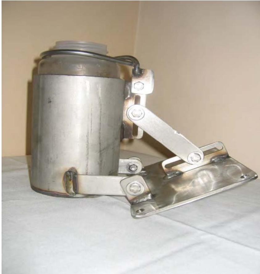
**Figure 8. Modified Ecology Sediment Trap**
