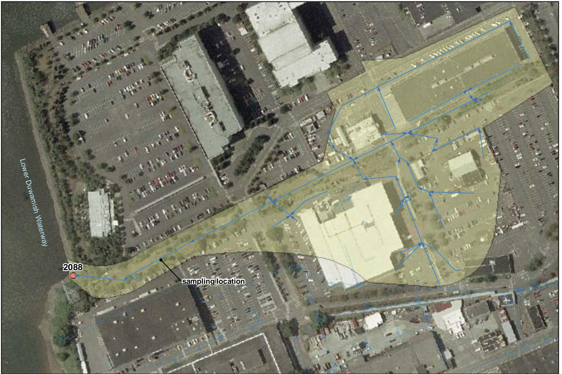
Figure 5. Boeing Developmental Center Storm Drain Basin and Outfall Location
