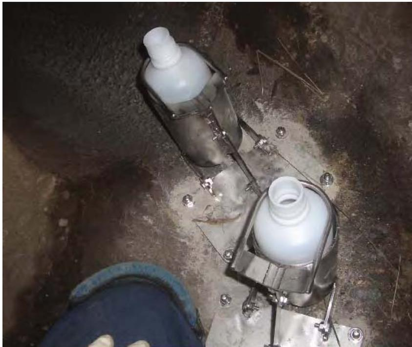
**Figure 9. Sediment Traps Installed
