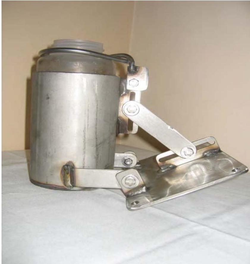
**Figure 6. Modified Ecology Sediment Trap**
