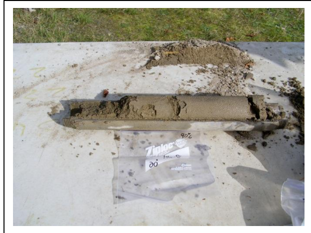
MW-8: Sample from 20-21.5 bgs – Poorly-Graded Sand (SP) Gray-Brown, moist to wet, mostly medium sand with trace gravel and trace silt. Photo by EPI.
