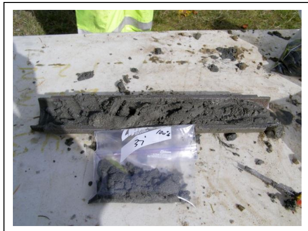
MW-8: Sample from 37-38.5 ft. bgs – Poorly-Graded Sand (SP) Wet, Grades to well-rounded medium sand with black, gray, and white grains. Photo by EPI.
