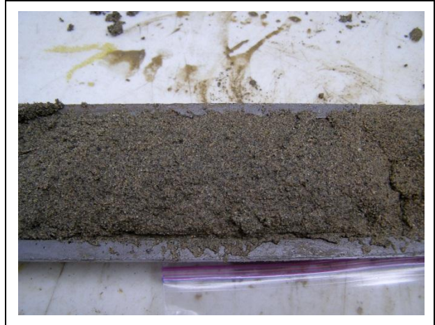
MW-10: Sample from 45-46.5 ft. bgs – Poorly Graded Sand (SP) Gray-Brown, Wet, mostly medium sand with trace gravel and trace silt. Photo by EPI.
