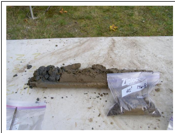
MW-8: Sample from 25-26.5 ft. bgs – Poorly Graded Sand (SP) Gray-Brown, moist to wet, mostly medium sand with trace gravel and trace silt. Photo by EPI.
