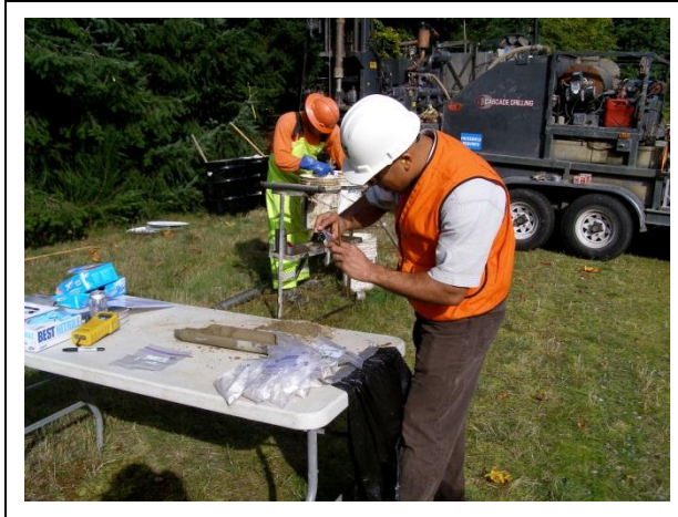
MW-8: Sample from 20-21.5 ft. bgs – Poorly-Graded Sand (SP) Gray-Brown, moist to wet, mostly medium sand with trace gravel and trace silt. Photo by EPI.
