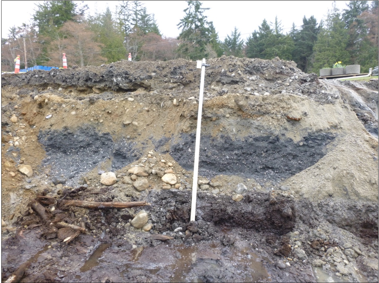
Figure 4-1 Southeastern AI showing layered terrestrial fill on top, marine fill dredge, and native peat on bottom, view south.
