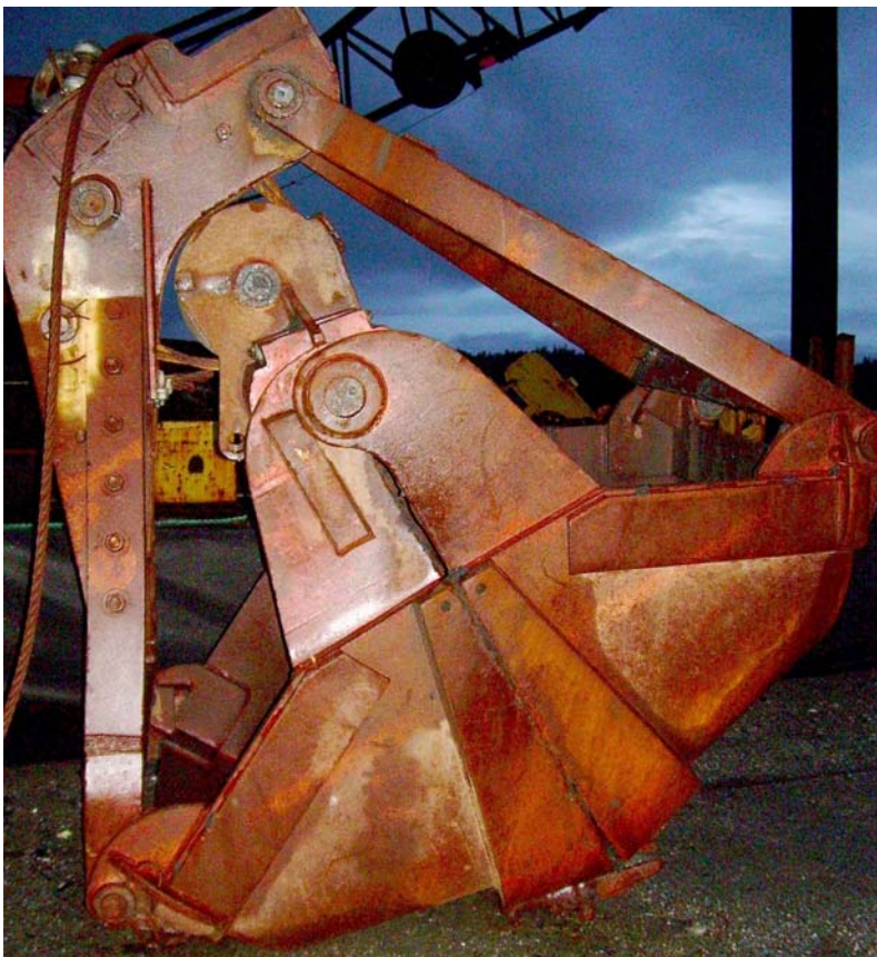
Photograph 2 - Dredge bucket (approximately 3 to 3.5 cubic yard volume).
