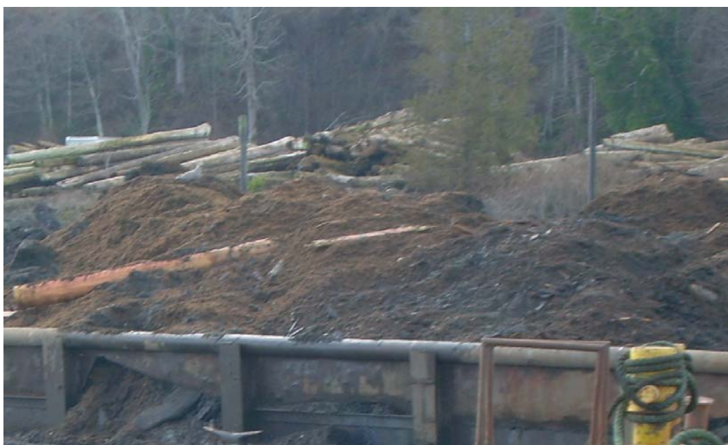
Photograph 5 - Example of sawdust-like dredged material (left) and silty, sandy woodwaste (right) on barge.
