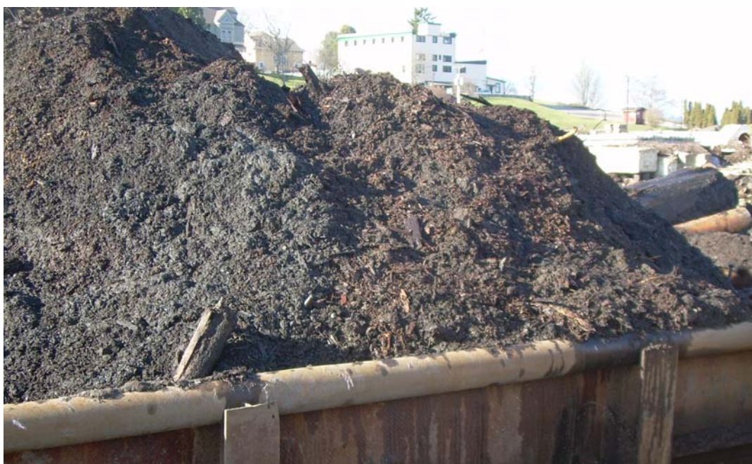
Photograph 8 - Dewatered sandy sediment on barge containing more wood material and less silt.
