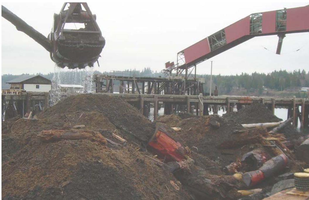
Photograph 4 - View of sawdust-like dredged material (light color), heterogeneous sediment/woodwaste (dark color), and large wood debris.
