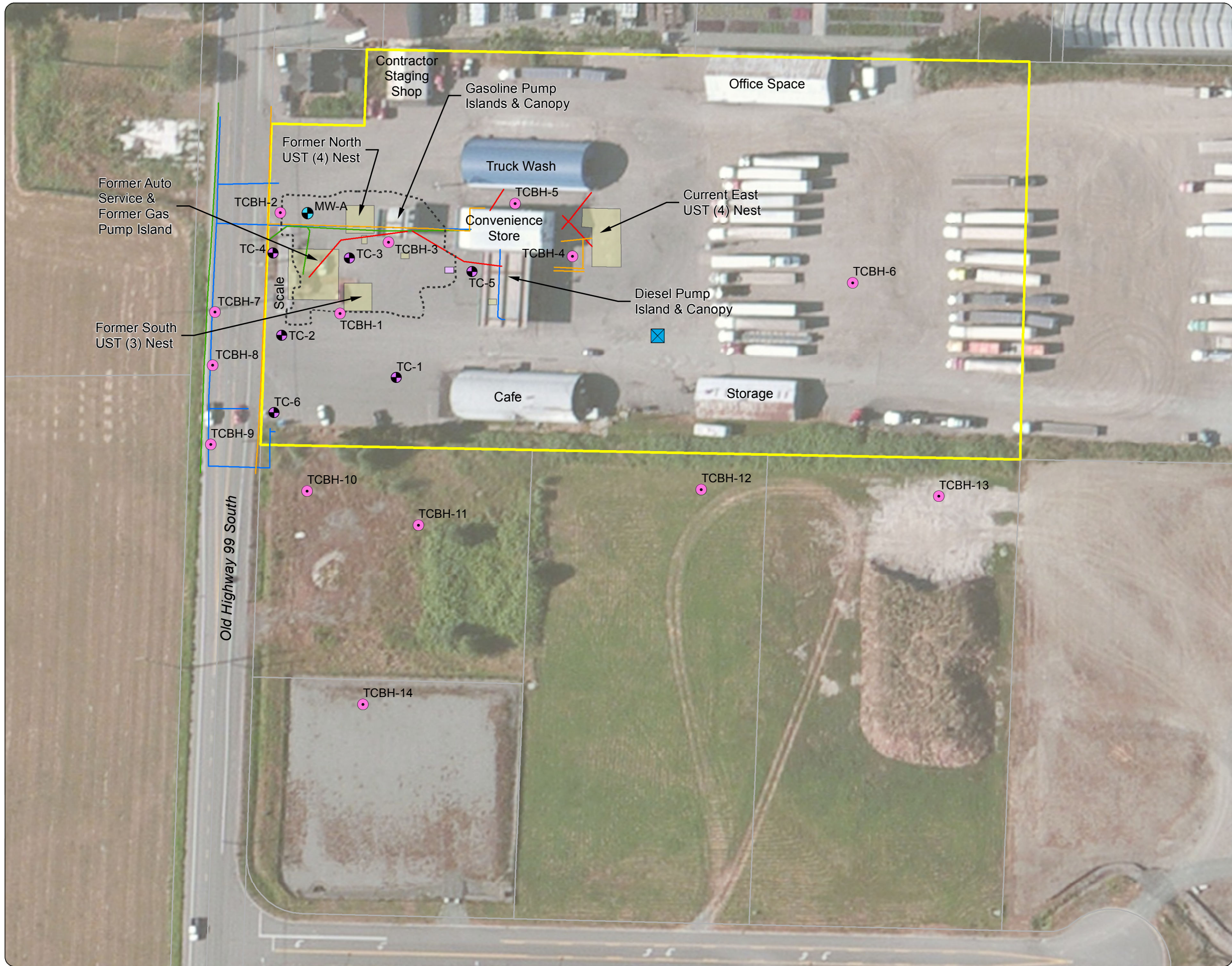
Figure 4 Site Features and Locations of Investigations
