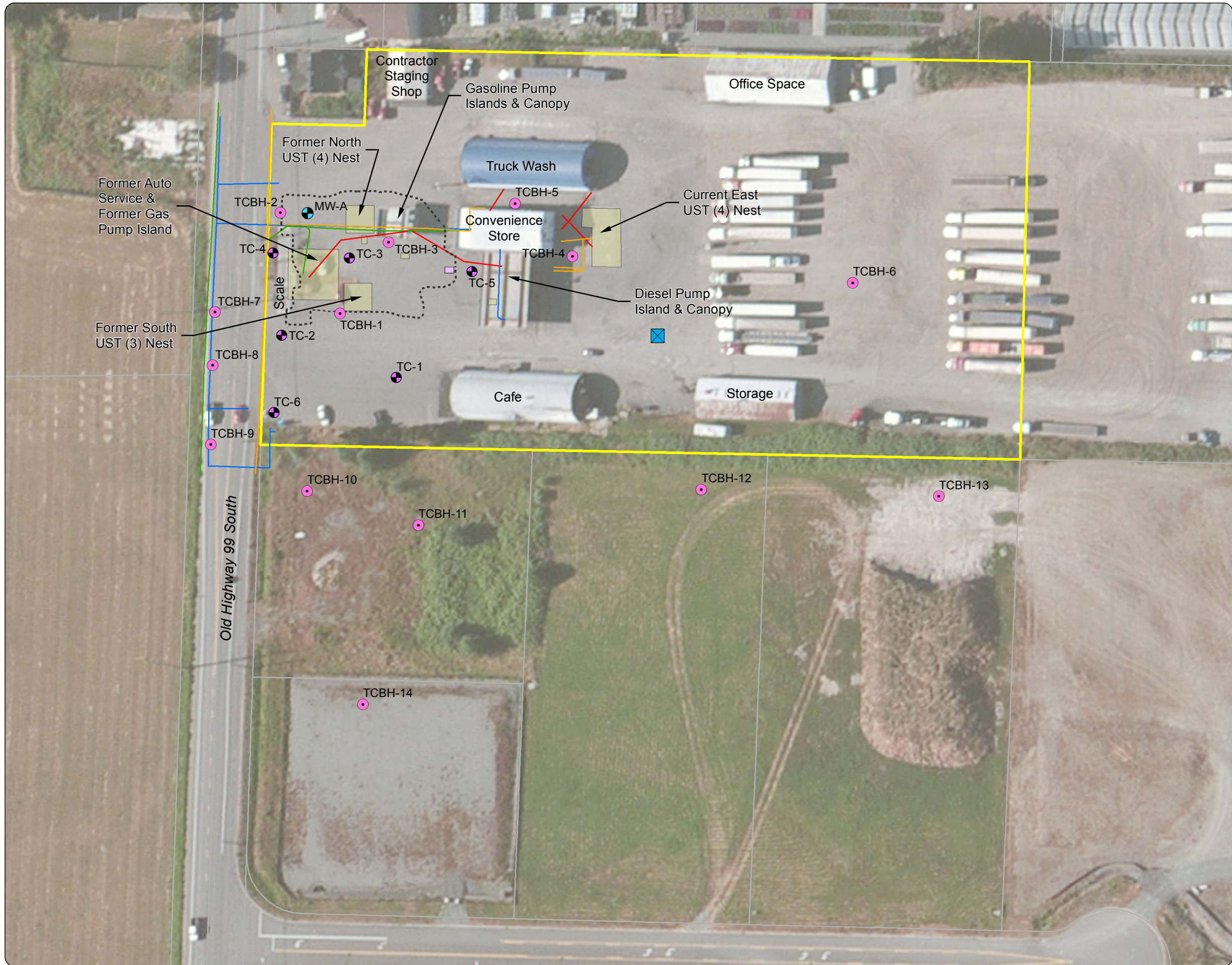
Figure 4 Site Features and Locations of Investigations
