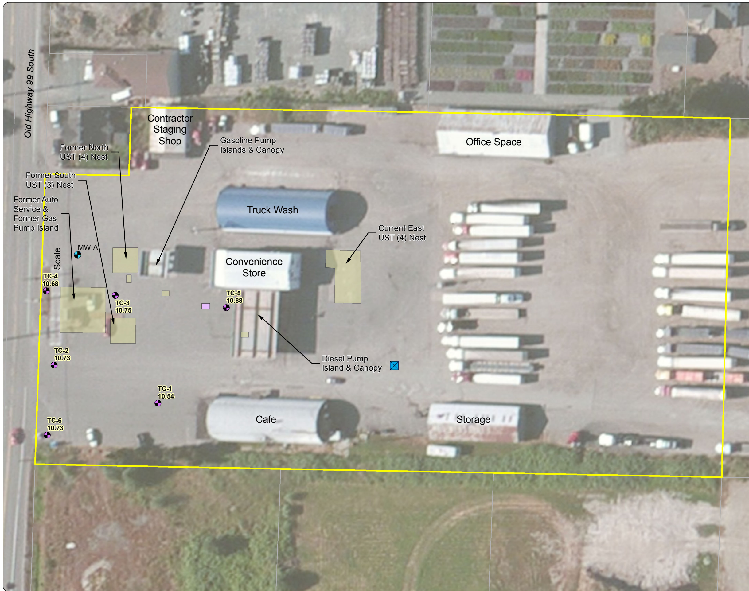
Figure 11 Compliance Monitoring Well Network
