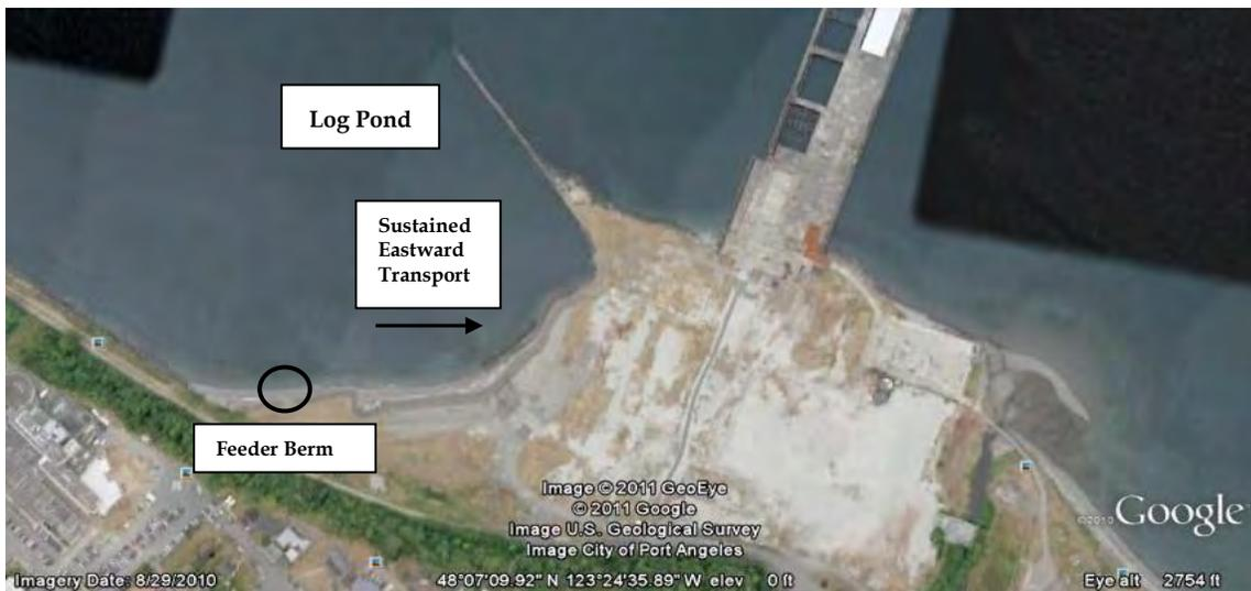
**Figure C.2-10. Log pond at the former Rayonier mill showing beach accretion east of the feeder berm**
