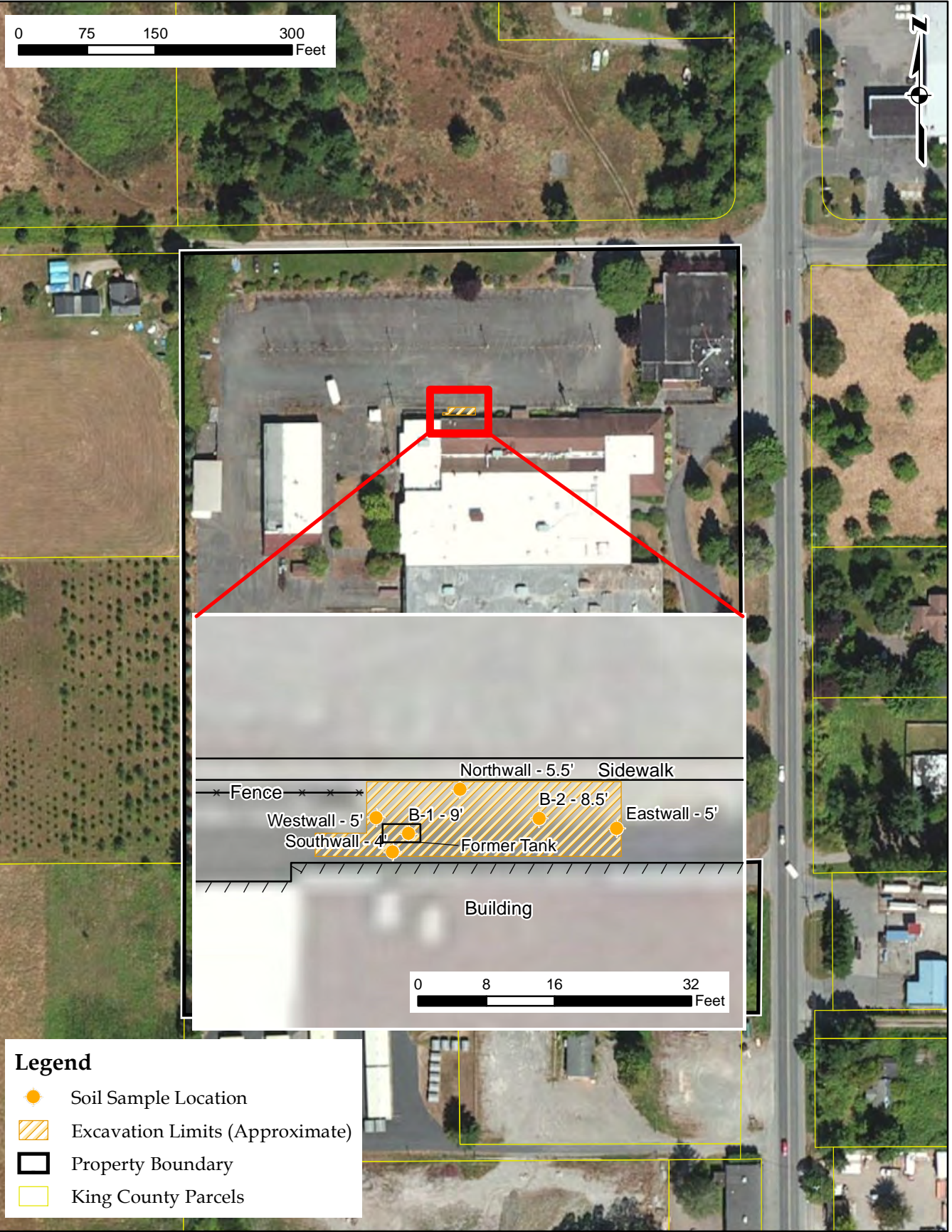
Figure 3 Underground Storage Tank Decommissioning K2 Site Investigation Vashon, Washington
