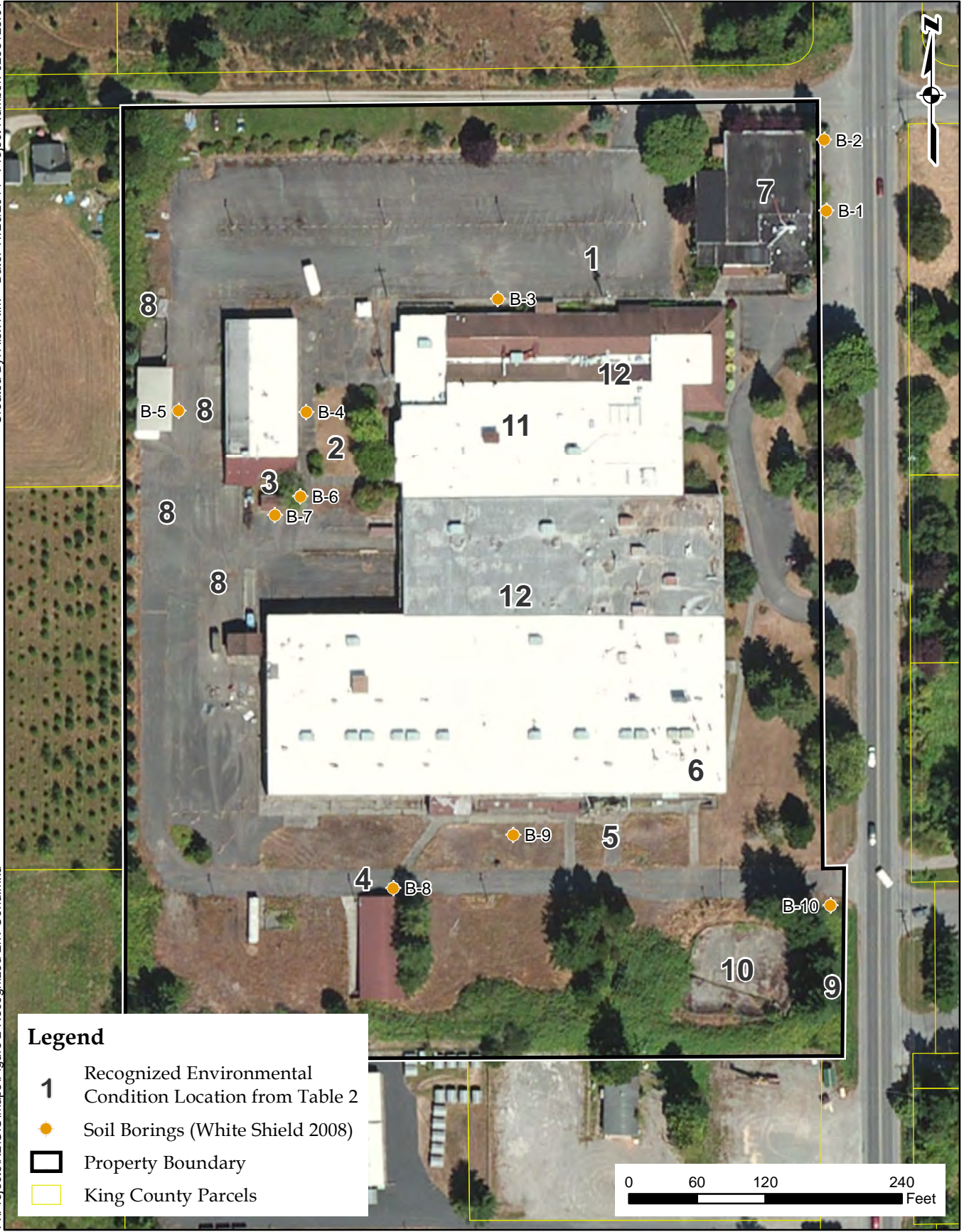
Figure 2 Recognized Environmental Condition Locations K2 Site Investigation Vashon, Washington
