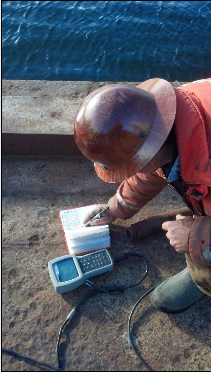
Photograph 5 – Contractor crew member taking manual background turbidity readings (February 7, 2014).
