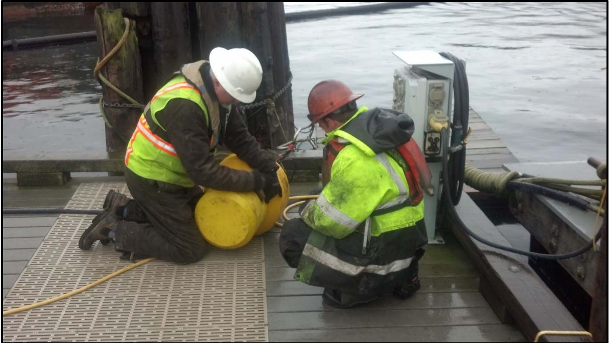
Photograph 24 – Contractor changing batteries on the water quality monitoring buoy (January 8, 2014).
