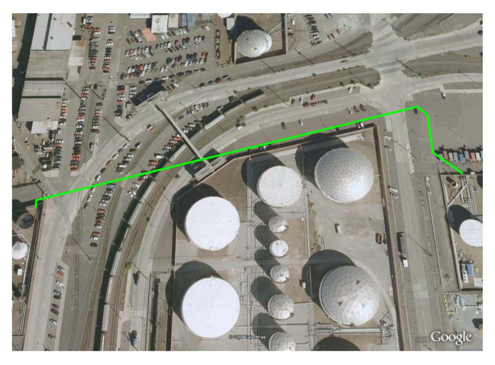
Approximate location of BP petroleum pipelines north of the Shell Terminal based upon a limited review of available drawings. Actual locations likely vary from those listed. This figure should not be interpreted as fact and the BP Seattle Terminal should be contacted to verify pipeline locations prior to initiating any ground disturbance activities near these lines. TechSolv assumes no responsibility for the information provided on this figure.
